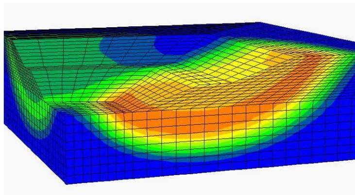
Figure 5: Contour of displacements ( $\Phi_u = 3^\circ$ ,  $C_u = 35$  kPa)
