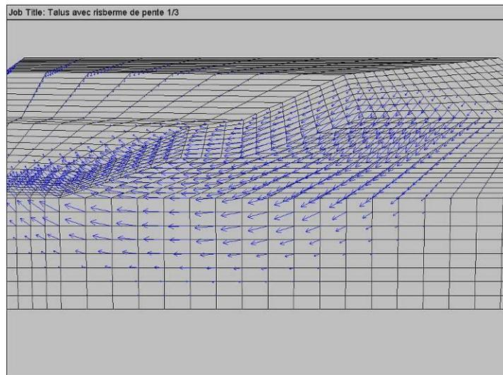
Figure 4. Vectors of displacements ( $\Phi_u = 3^\circ$ ,  $C_u = 35$  kPa)
