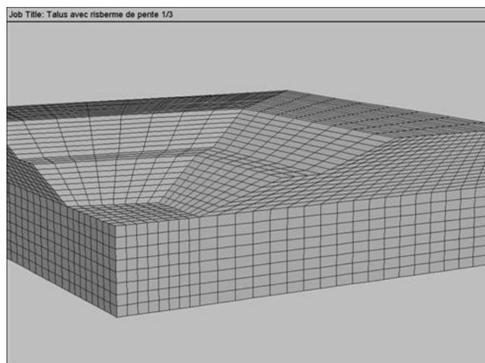
Figure 3. Mesh used 7808 elements and 9093 nodes (part of receptacle)
