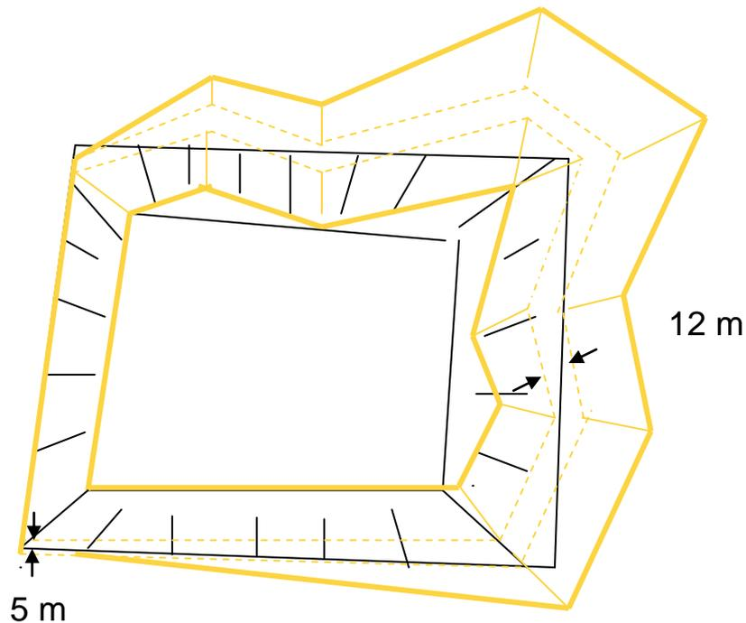
Figure 2. Superposition of the new form of receptacle with the old (solution with berm)
