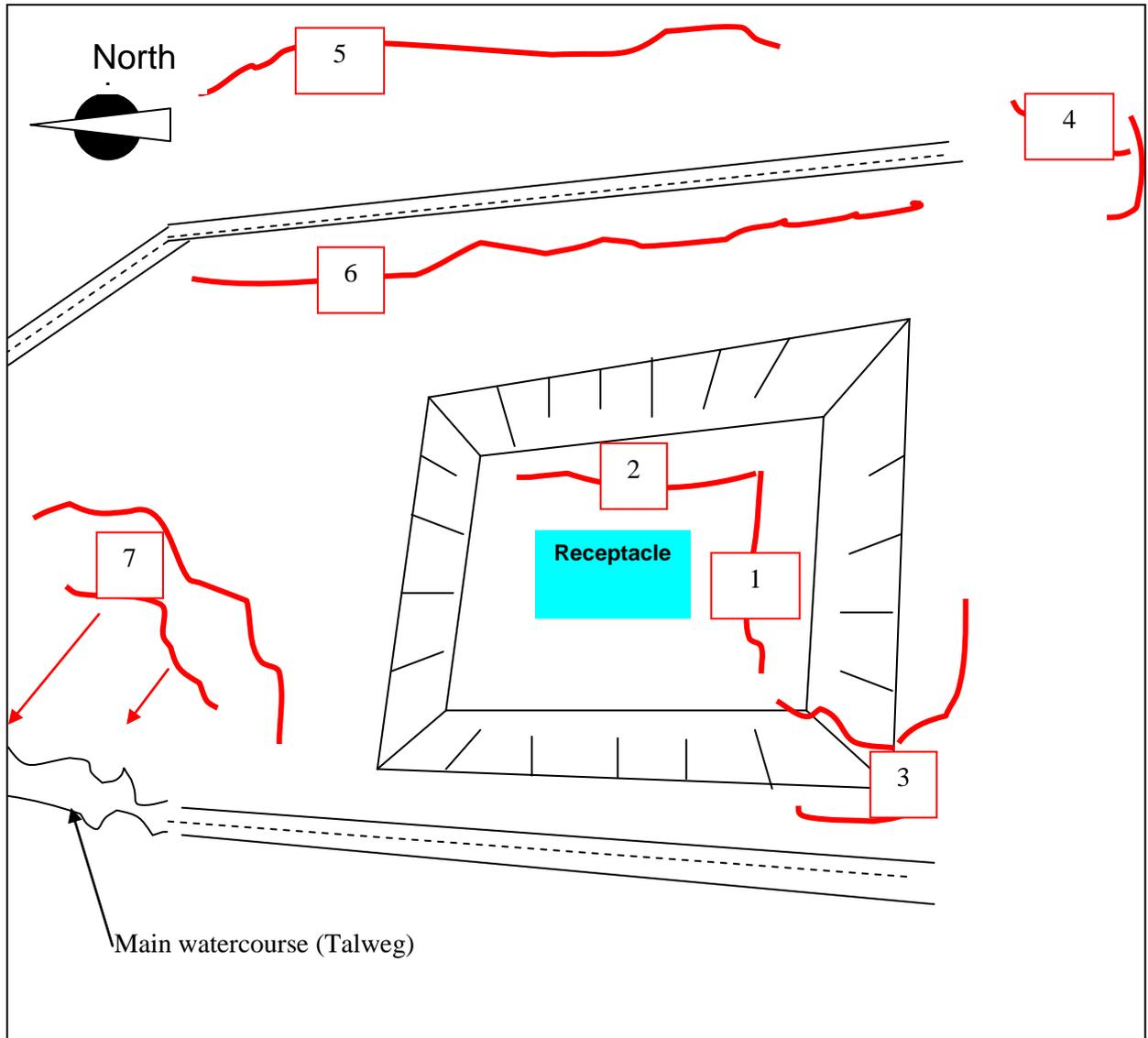
Figure1. Schematic of the receptacle and cracks observed
