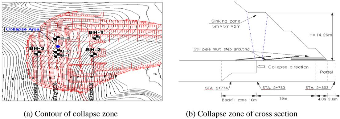
Figure 4. Ground profile and tunnel cross section
