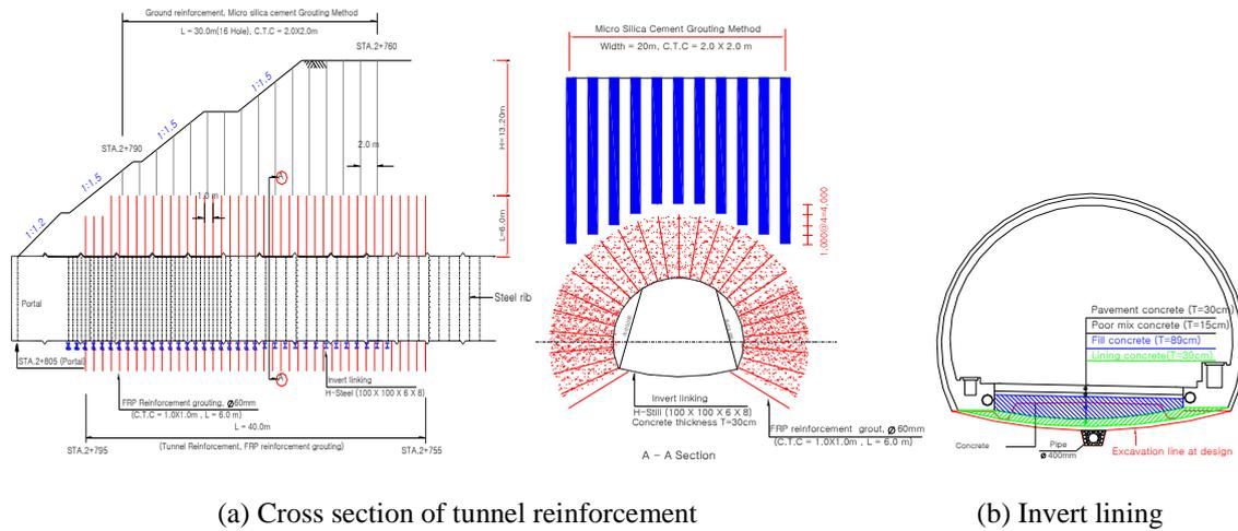
Figure 6. Reinforcement of collapsed area
