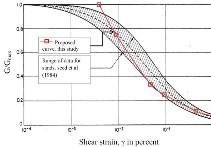
Figure 1. Comparison of the proposed equation (3) in this study and range of data for sands defined by Seed et al. (1984).
