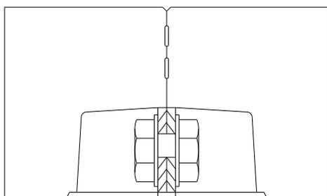
Figure 4. Box bolt fastening method
