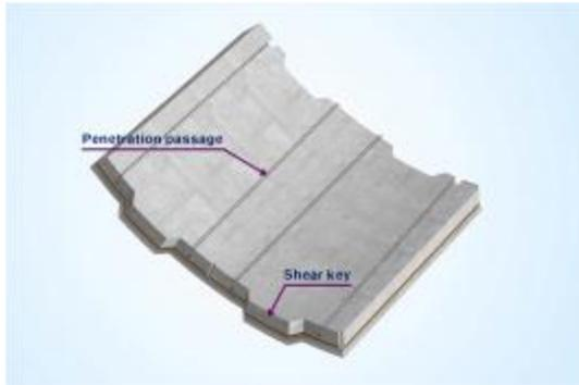
Figure 11. Segment cross-section schematic diagram
