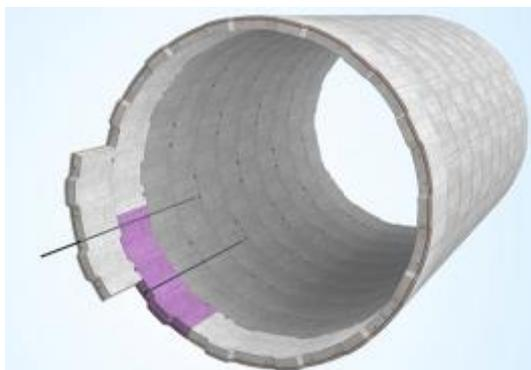
(c) Additional installation of lateral segment
