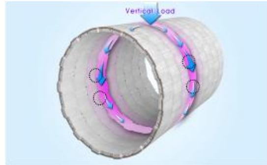
Figure 12. Stress redistribution through shear keys
