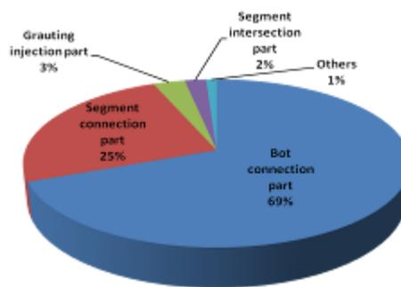
Figure 1. Distribution of leakage occurred in the segment tunnel
