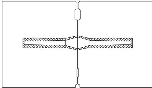
Figure 6. Pin fastening method
