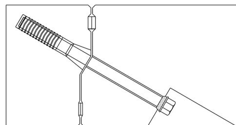
Figure 5. Inclined bolt fastening method
