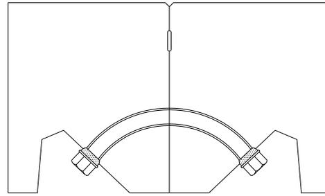
Figure 7. Bent bolt fastening method
