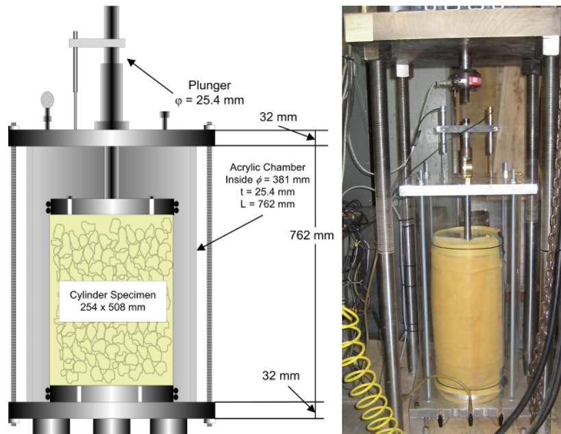
Figure 5: Triaxial chamber used for specimen with nominal dimensions 254-mm diameter x 508-mm height.
