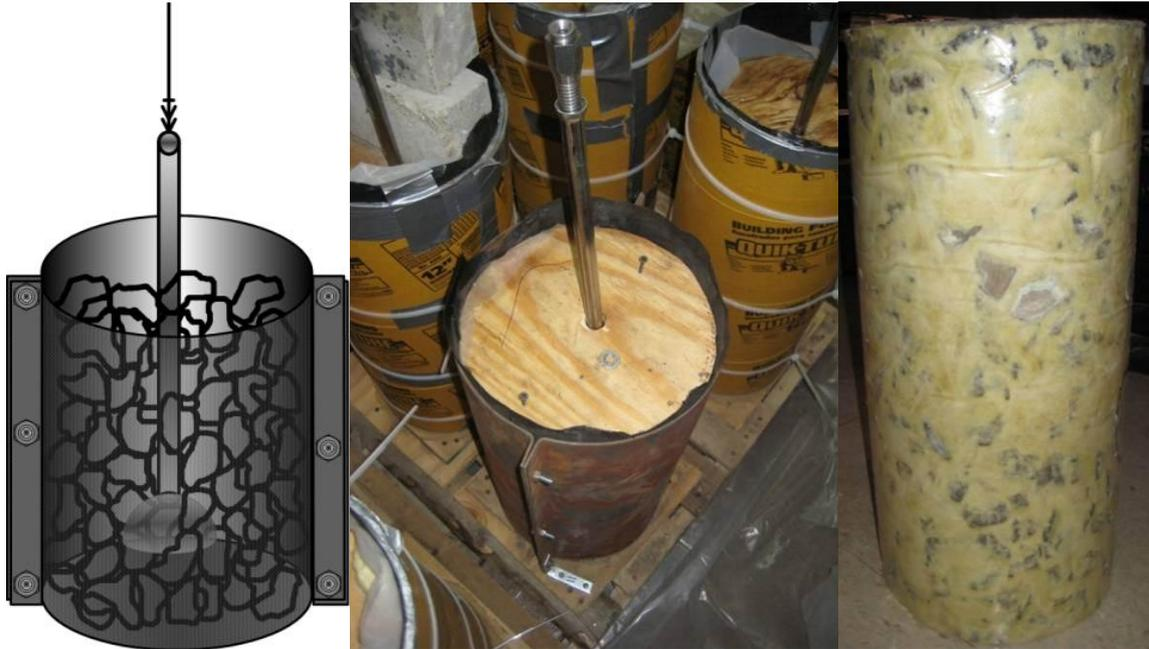
Figure 4: Diagram of injection mold (left), picture of specimen fabrication molds (middle), picture of PSB cylindrical specimen (right)
