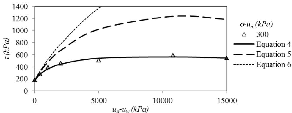
Figure 2. Comparison of predicted and experimental shear strength of Madrid gray clay, using different formulae for large suction range under a single net normal stress.
