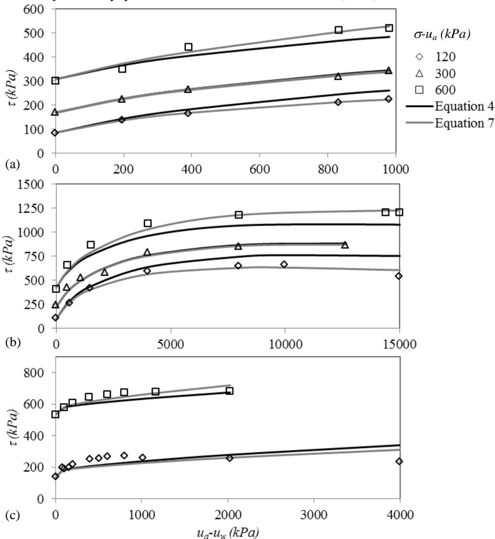
Figure 5. Comparison of accuracy of the predicted shear strength using equation 4 and 7 for different net normal stresses on: (a) Gray clay (Experimental data from Escario and Saez, 1986); (b) Red clay and (c) Clayey sand (Experimental data from Escario and Juca, 1989).
