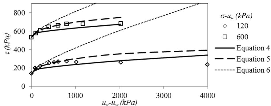
Figure 4. Comparison of predicted and experimental shear strength of Madrid clayey sand, using different formulae for large suction range under two different net normal stresses.
