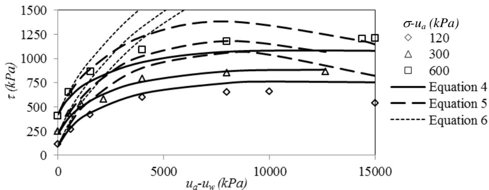
Figure 3. Comparison of predicted and experimental shear strength of Red clay, using different formulae for large suction range under three different net normal stresses.
