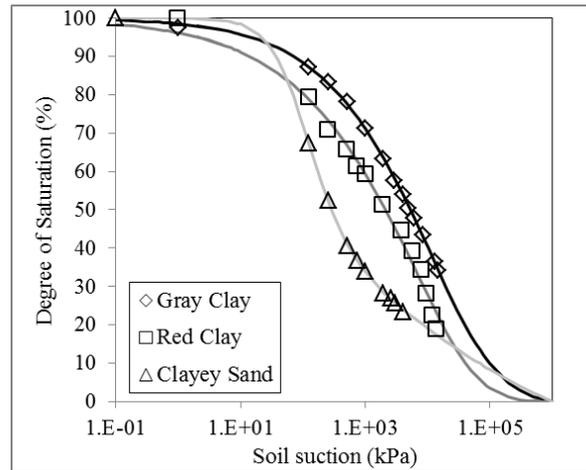
Figure 1. Soil-water characteristic curves for three soils tested by Escasrio and Juca (1989).
