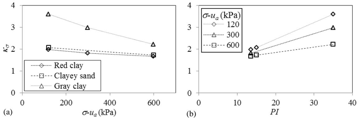
Figure 6. Variation of  $\kappa_\sigma$  with respect to: (a) net normal stress and (b) PI.
