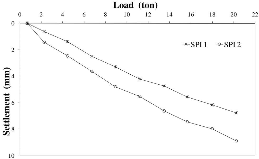
Figure 1 Load deformation curves for Single Pier Impact (SPI) columns (Kurt, 2011).
