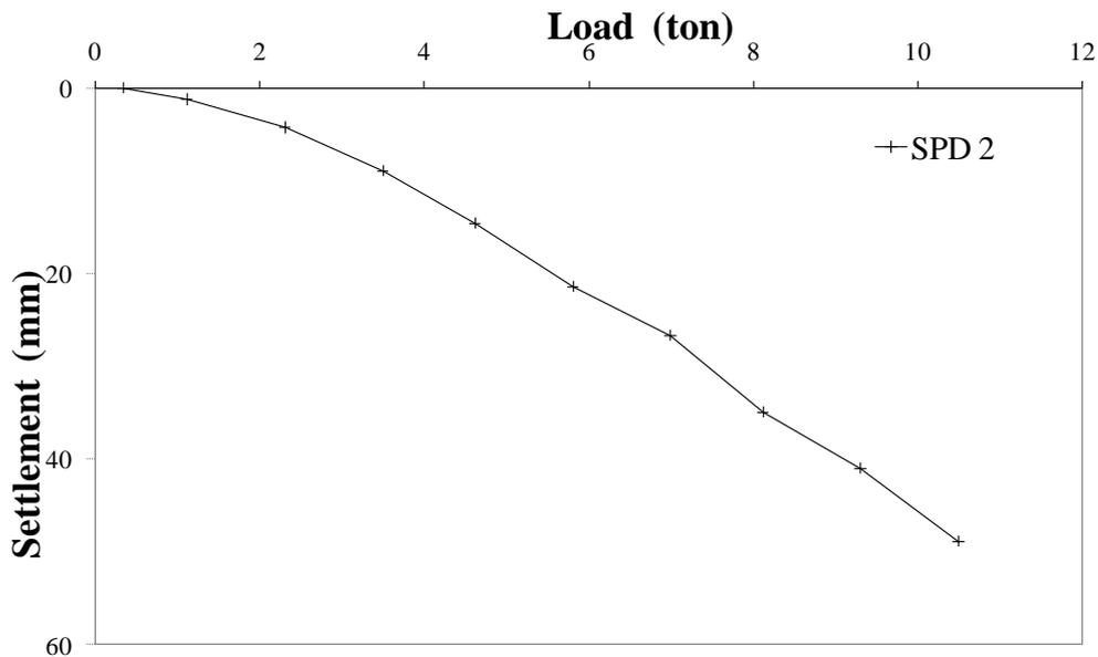
Figure 2 Load deformation curve for Single Pier Displacement (SPD) column (Kurt, 2011).
