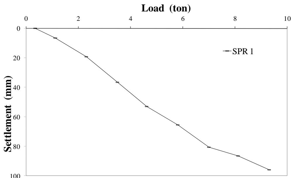
Figure 3 Load deformation curve for Single Pier Replacement (SPR) column (Kurt, 2011).
