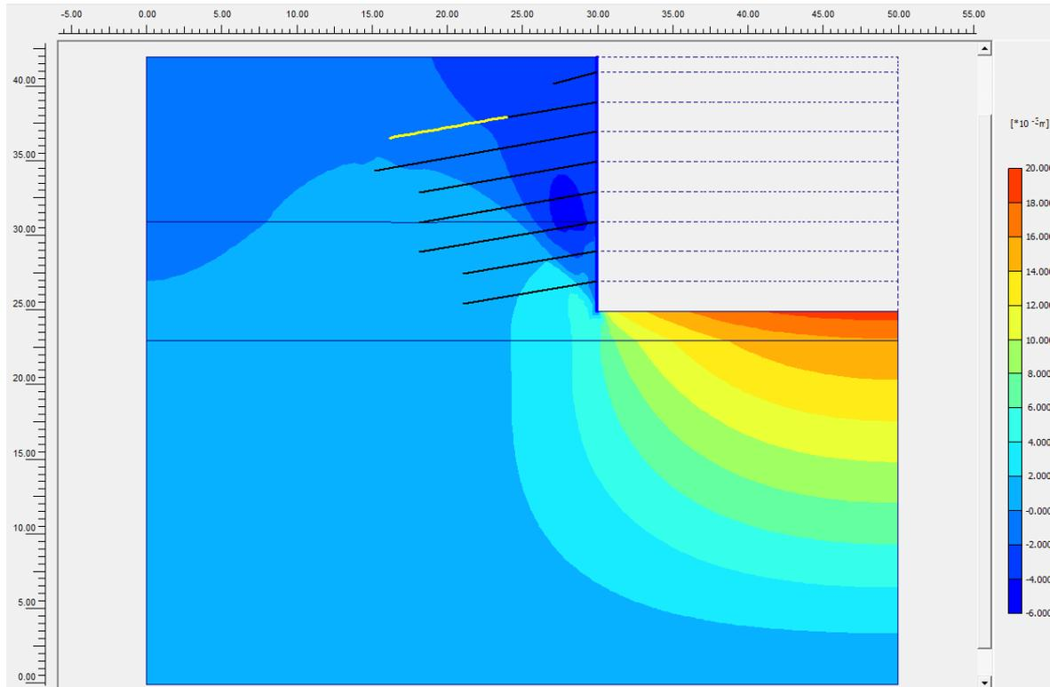
Figure 3. PLAXIS results (vertical displacements) for East wall
