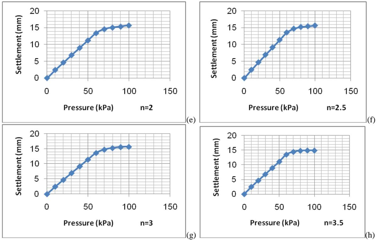
Figures 5. Pressure-settlement curves for models with various ratio of  $n = H/D$ .
