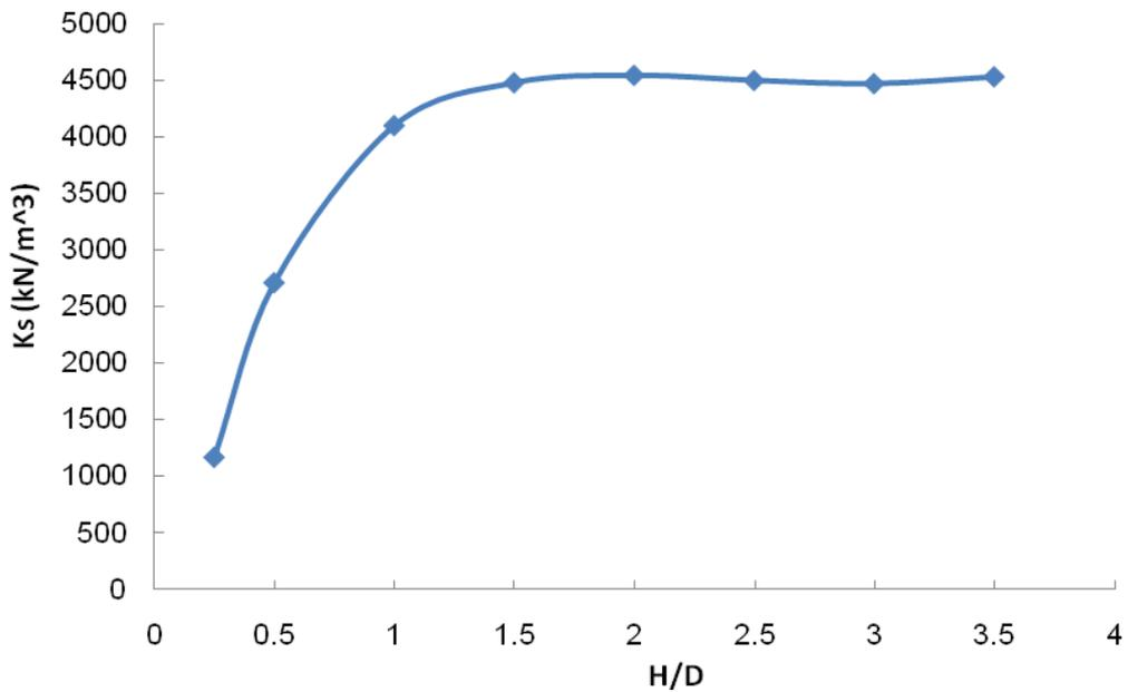
Figure 6. Subgrade reaction modulus for different ratio of  $H/D$ .
