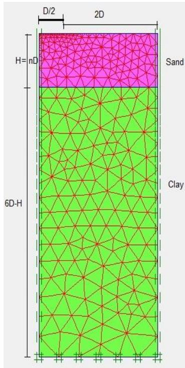
Figure 2. Model geometry.
