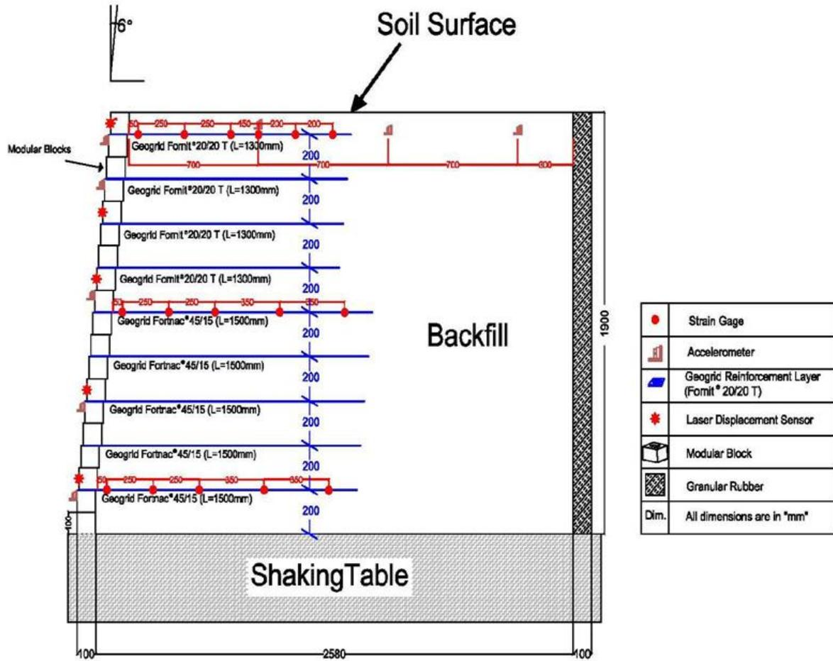
Figure 1. Schematic view of the model wall and locations of instrumentations.
