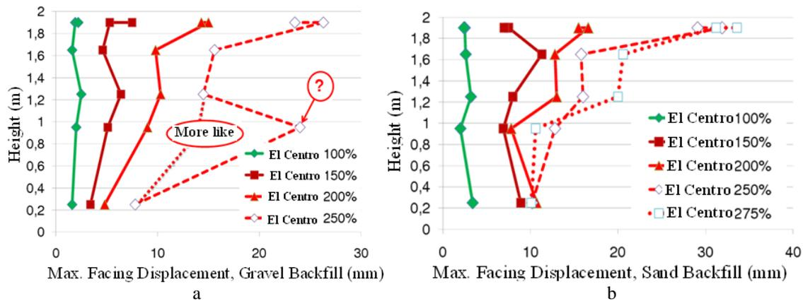
Figure 9. Facing displacement along the height of Walls under El Centro Earthquake with different intensities: a. Wall 1 (Gravel), b. Wall 2 (Sand).
