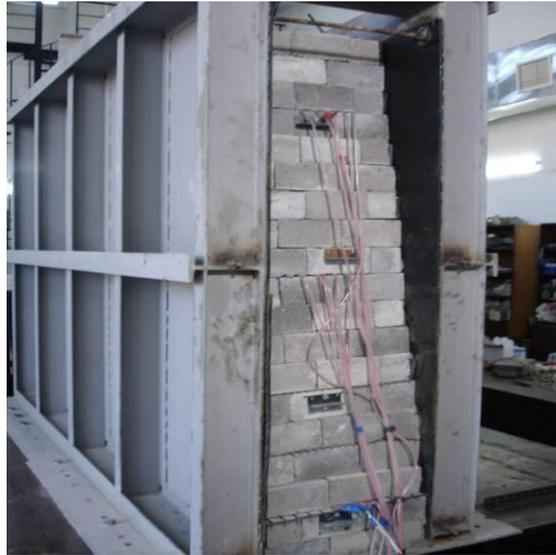
Figure 2. An overall view of the model wall with accelerometers and strain gages mounted
