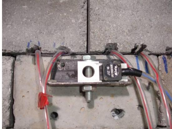
Figure 5. One of the accelerometers mounted on block facing and strain gage cables.
