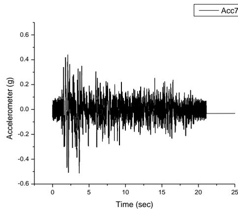
Figure 6. The 100% El-Centro Earthquake Record.
