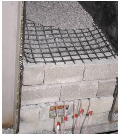
Figure 3. Installation of geogrids with frictional connection to the facing blocks.
