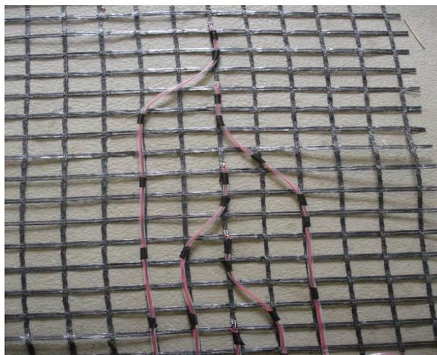
Figure 4. Strain gage setup on geogrid.
