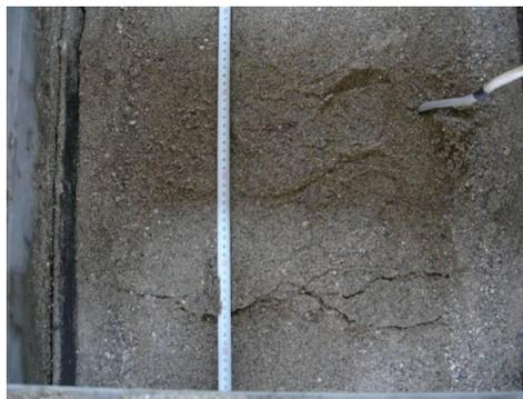
Figure 8. Tensile cracks observed in sand backfill behind the reinforced zone.
