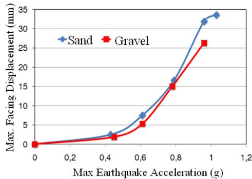
Figure 7. Maximum horizontal facing displacements vs. maximum seismic accelerations.
