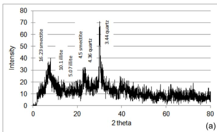
Figure 2. Semi-quantitative XRD scan representing the peaks of clay components
