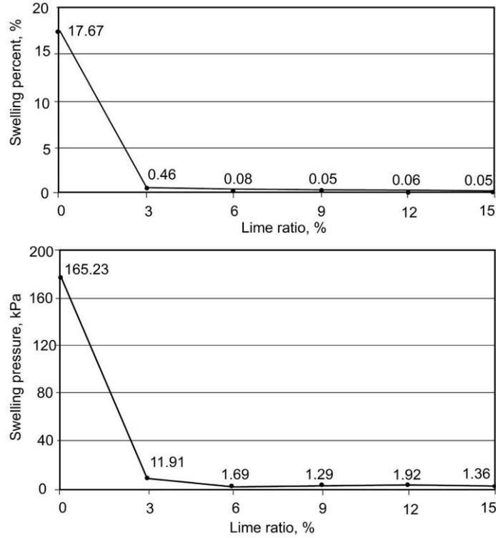
Figure 3. Lime ratio vs. swelling percent and swelling pressure at 90 days
