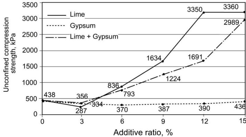
Figure 6. Additives vs. unconfined compression strength
