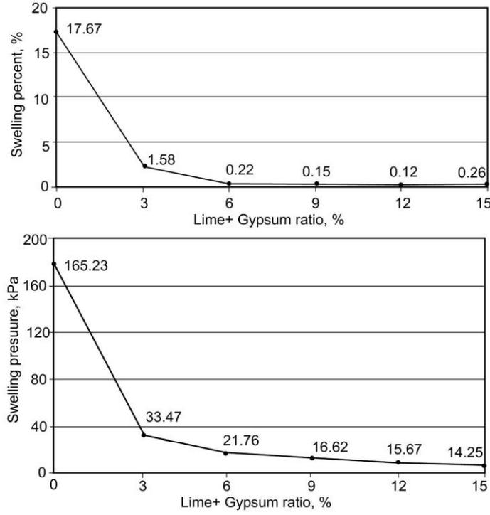
Figure 5. Lime + Gypsum ratio vs. swelling percent and swelling pressure
