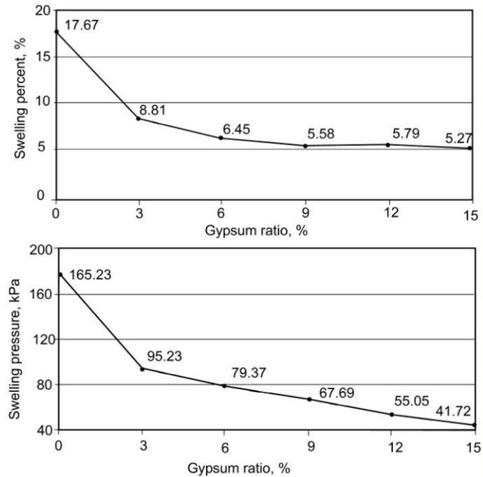
Figure 4. Gypsum ratio vs. swelling percent and swelling pressure at 90 days
