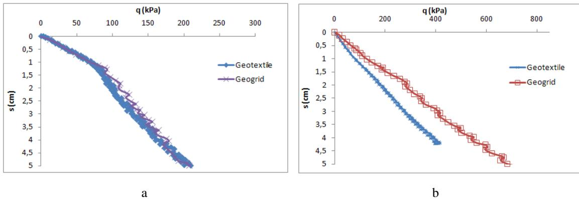
Figure 4. Comparison of geotextile and geogrid reinforced soil; a.  $N=1$ ,  $b=N=3$ .
