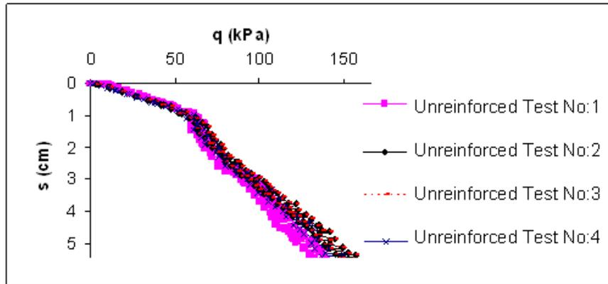
Figure 2. Load-settlement curves for strip footing on unreinforced sand.
