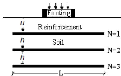
Figure 1. Schematic of reinforced soil model.
