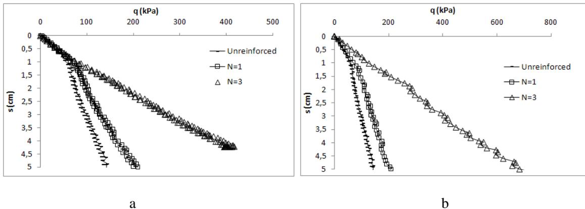
Figure 3. Load-settlement curves for strip footing on reinforced sand; a. geotextile, b. geogrid reinforced.
