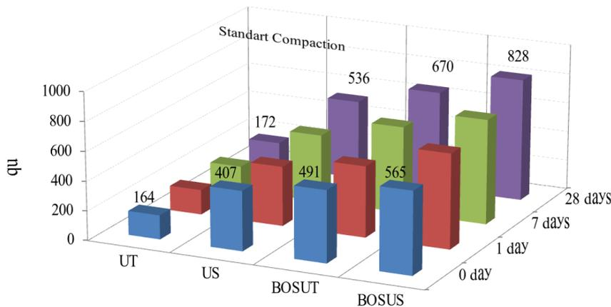
Figure 2. Variation of  $q_u$  values of the samples at 0, 1, 7 and 28 days curing periods.
