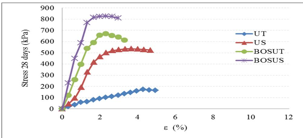
Figure 4. Typical stress–strain behavior of the samples at 28-day curing periods in UC tests.
