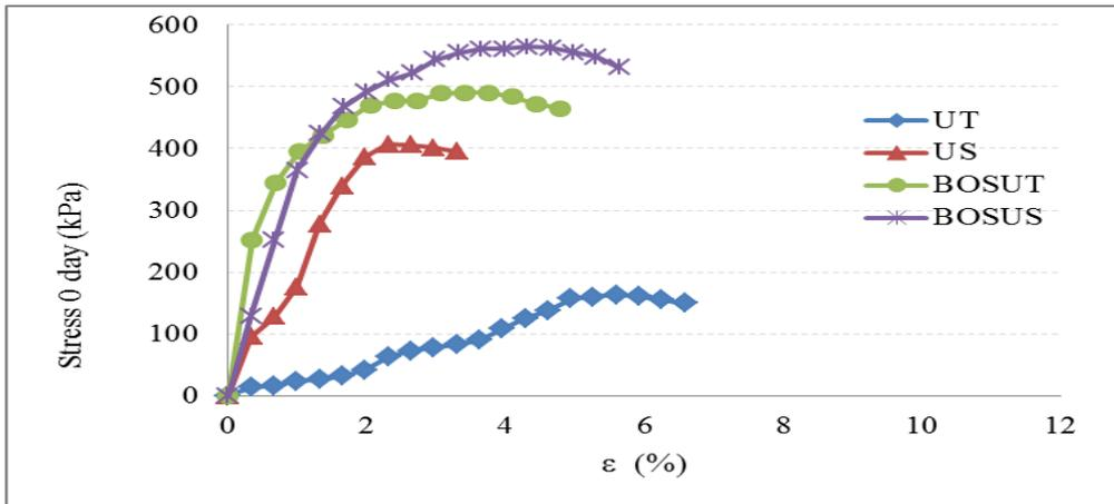
Figure 3. Typical stress – strain behavior of the samples at 0-day curing periods in UC tests.
