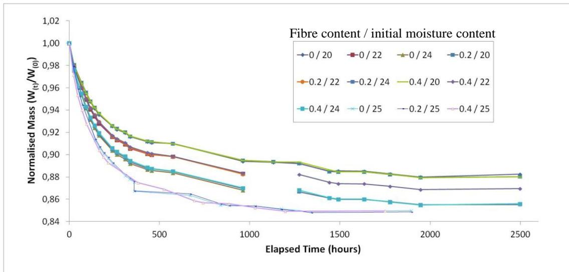
Figure 2. Change in normalised mass of reinforced and unreinforced samples due to free swell
