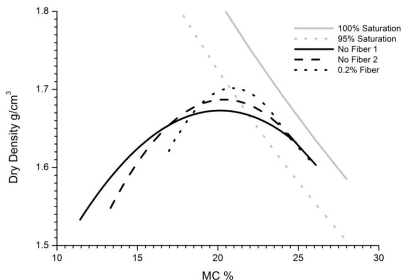
Figure 1. Compaction curves of reinforced and non-reinforced samples
