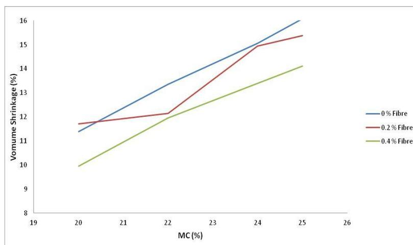
Figure 6. End of drying period volume of samples
