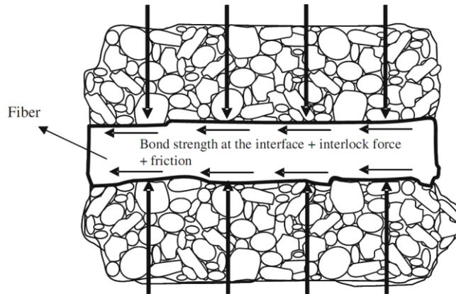
Figure 5. Schematic diagram of mechanical behaviour at the interface between fibre surface and soil particles (Tang et al. 2007).
