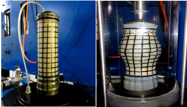
Figure 3. Examples of a prepared triaxial sample prior to testing and a deformed specimen after testing
