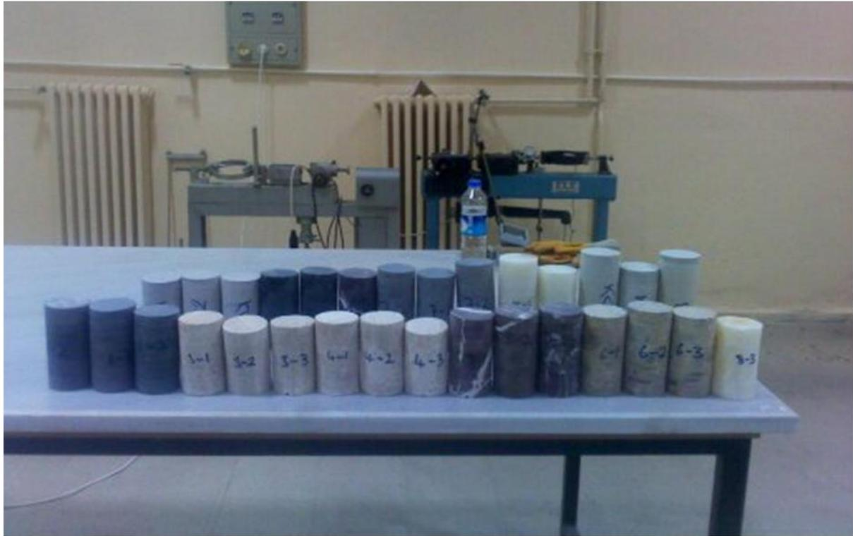
Figure 2. Core samples before uniaxial compression test.
