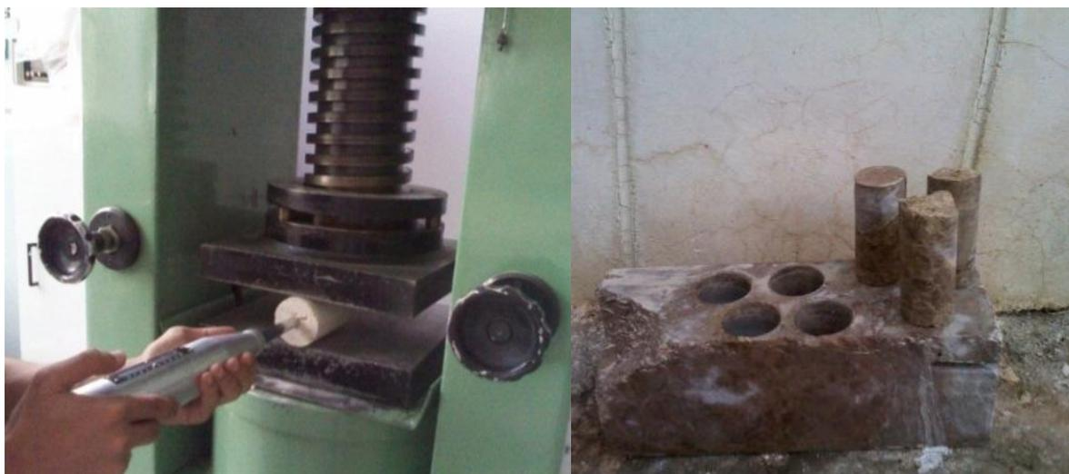
Figure 1. Schmidt tests and core samples
