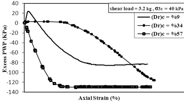
Figure 4. Excess pore water pressure versus axial strain at different relative densities and small shear load in anisotropic stress condition
