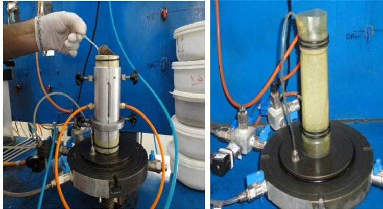
Figure 2. Examples of a procedure and prepared triaxial sample
