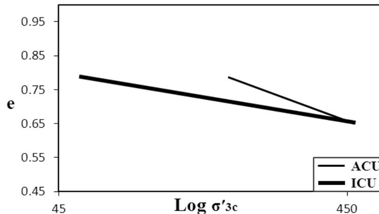
Figure 13. CVR lines at Anisotropic (ACU) and Isotropic (ICU) conditions with different relative densities for Babolsar clean sand
