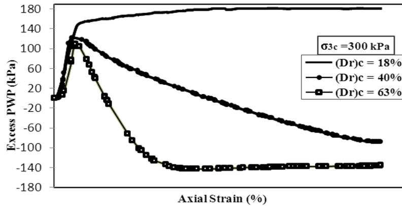
Figure 10. Excess pore water pressure versus axial strain at different relative densities and high effective confining pressure in isotropic stress condition
