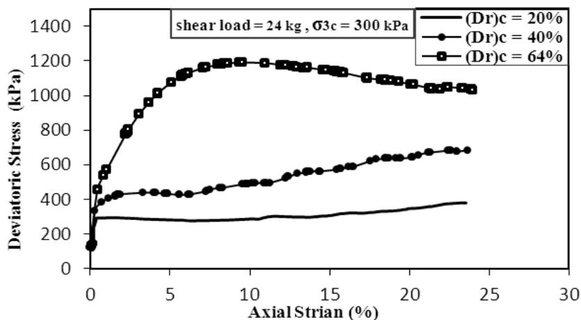
Figure 8. Stress-strain behavior at different relative densities and high shear load in anisotropic stress condition
