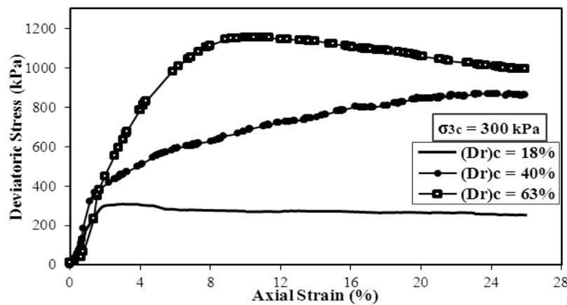
Figure 11. Stress-strain behavior at different relative densities and high effective confining pressure in isotropic stress condition
