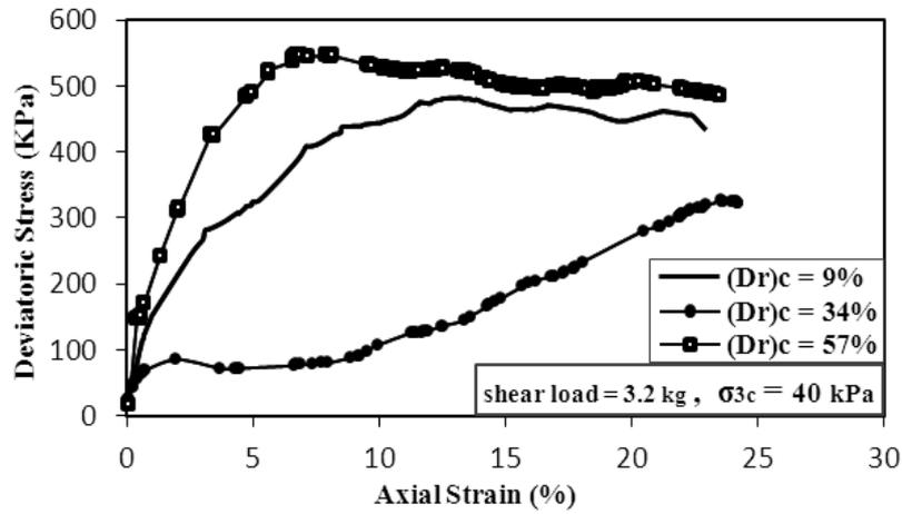
Figure 5. Stress-strain behavior at different relative densities and small shear load in anisotropic stress condition
