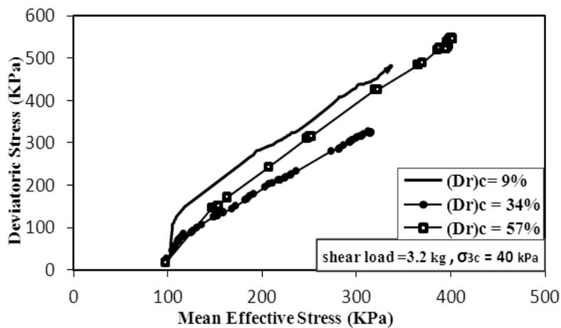
Figure 6. Effective stress path at different relative densities and small shear load in anisotropic stress condition
