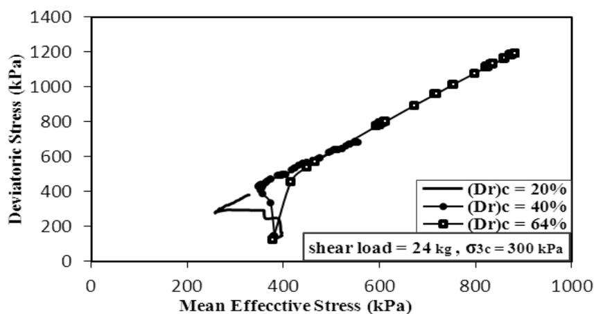
Figure 9. Effective stress path at different relative densities and high shear load in anisotropic stress condition
