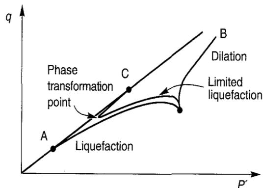
Figure 1. Liquefaction, limited liquefaction, and dilation in monotonic loading tests (after Castro 1996)
