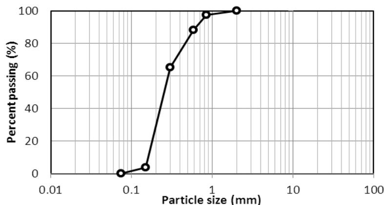
Figure 3. Grains size distribution curve for Babolsar sand
