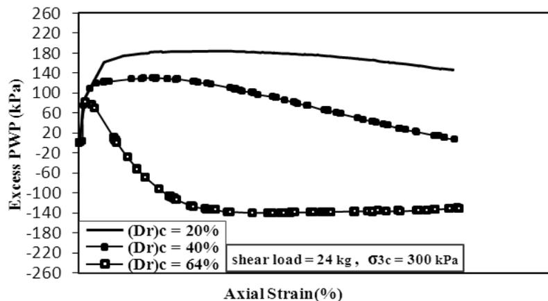
Figure 7. Excess pore water pressure versus axial strain at different relative densities and high shear load in anisotropic stress condition
