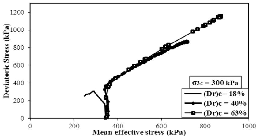
Figure 12. Effective stress path at different relative densities and high effective confining pressure in isotropic stress condition
