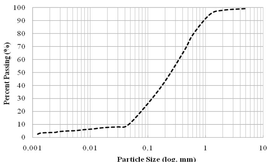
Figure 1. Grain-size distribution curve of the soil
