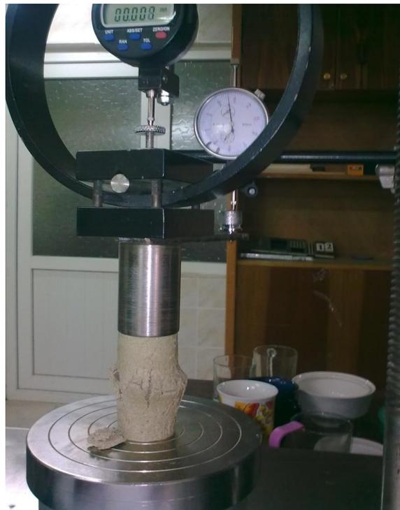
Figure 2. Unconfined compression testing device
