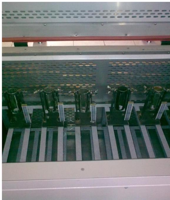
Figure 3. Freeze-thaw test under load (Special loading mechanisms and automatic freeze-thaw test cabin)
