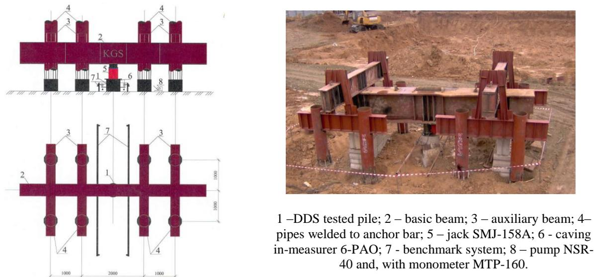
Figure 3. Static load test performance
