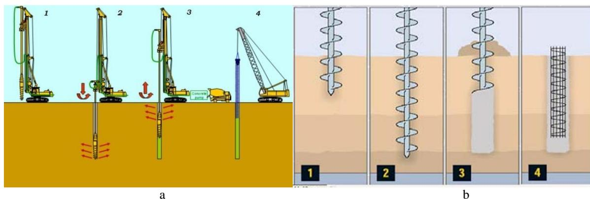
Figure 2. a) DDS and b) CFA pile installation.
