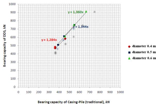
Figure 5. Comparison of DDS and Casing boring piles bearing capacities
