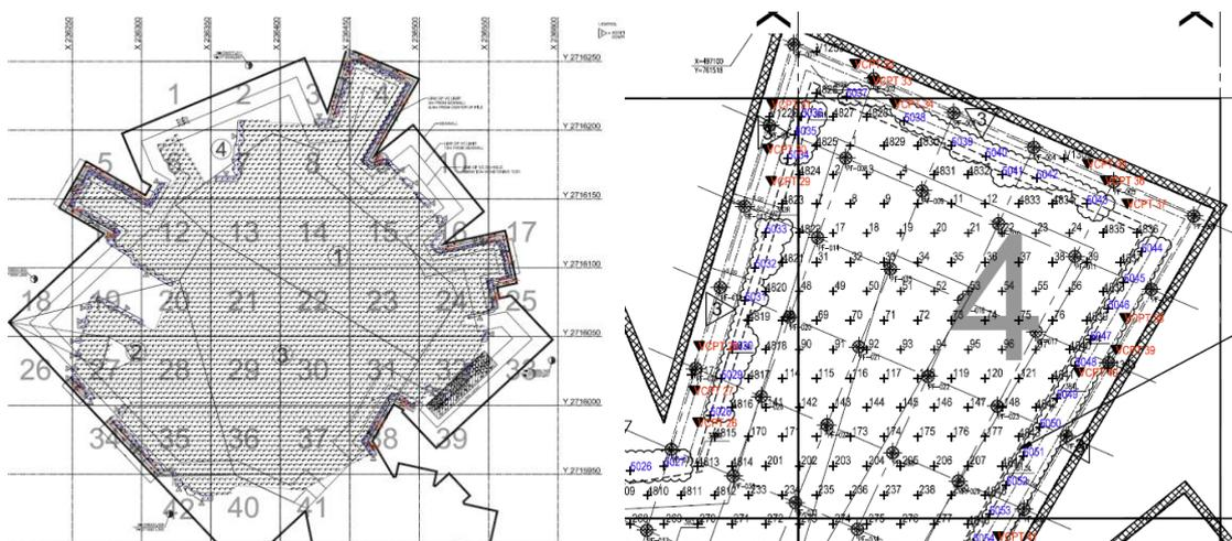
Figure 8. Layout of building with densification points (left),
