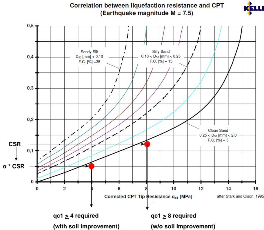
Figure 3. An example of reduction of the required cone penetration resistance  $q_c$  due to ground improvement (vibro replacement)
