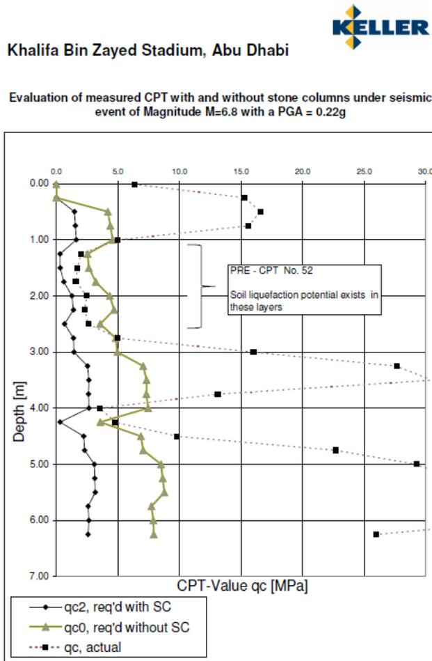
Figure 7. Cone penetration test including required tip resistance with and without vibro stone columns
