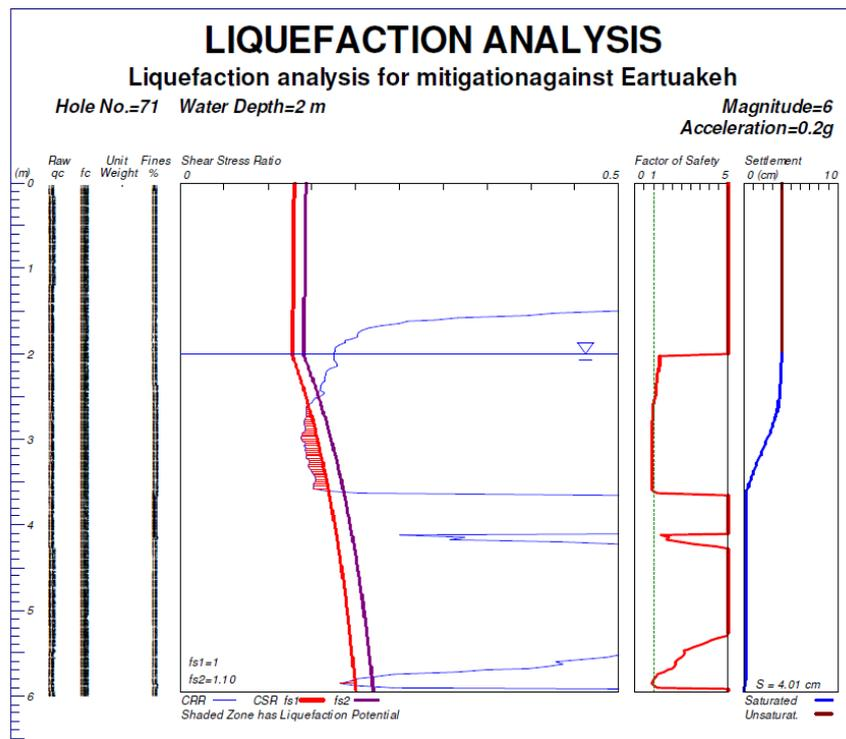
Figure 9. Liquefaction analysis (before densification)
