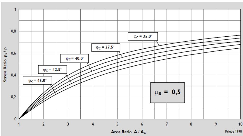
Figure 2. Reduction factor for the seismic stress ratio using vibro replacement (Priebe 1998)
