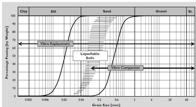
Figure 4. Application range of vibro compaction and vibro replacement methods by Priebe, 1998
