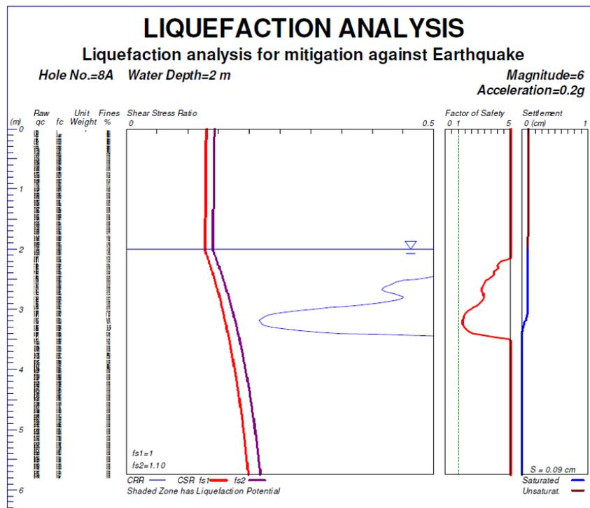
Figure 10. Liquefaction analysis (after densification)
