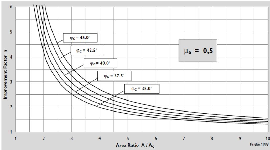
Figure 1: Design chart by Priebe, 1998 to calculate the soil improvement factor for settlements
