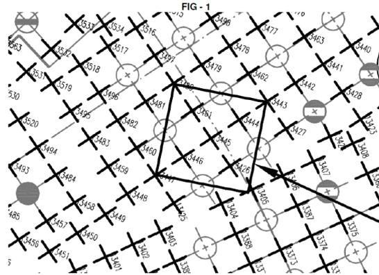
Figure 6. Typical arrangement of the vibro stone columns (crosses) around the bored piles (circles), with marked test field for load test
