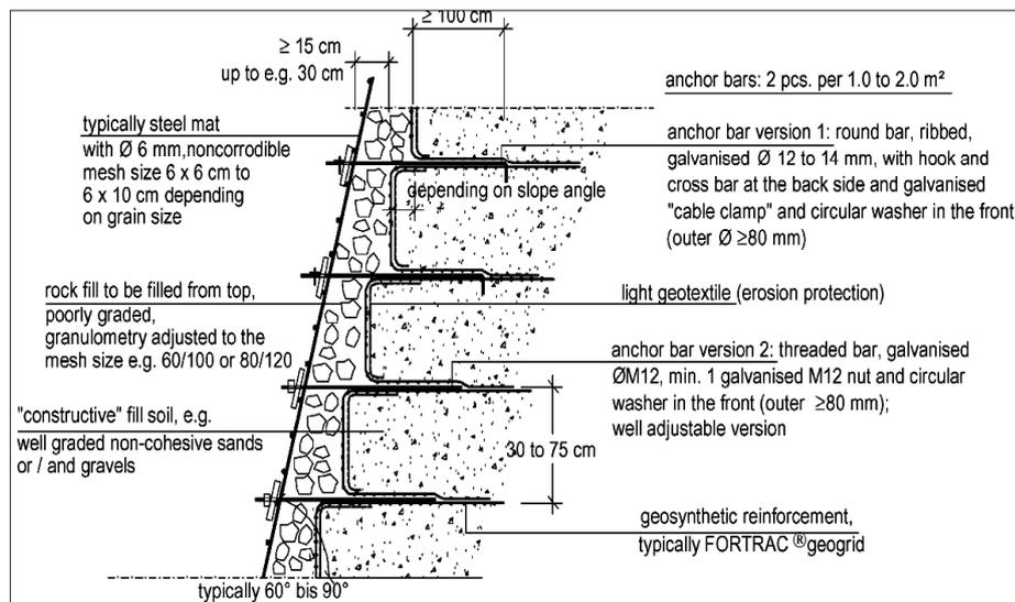
Figure 4. A typical version of the facing system Muralex®.
