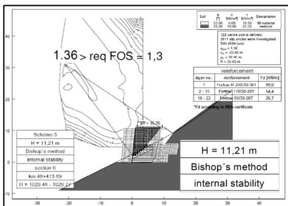
Figure 6. Typical example of stability analyses according to Bishop (only “internal” shown).
