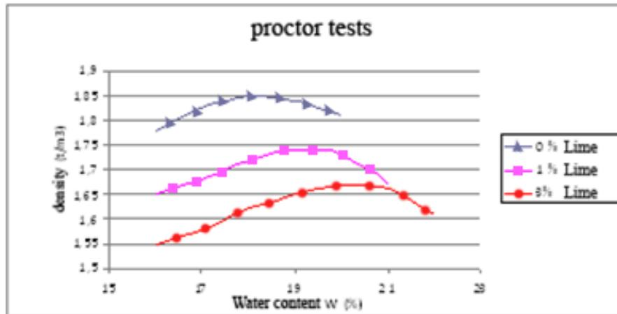
Figure 6. Proctor compaction test before and after treatment
