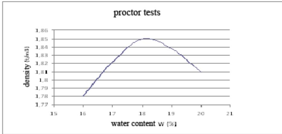
Figure 4. Proctor compaction test
