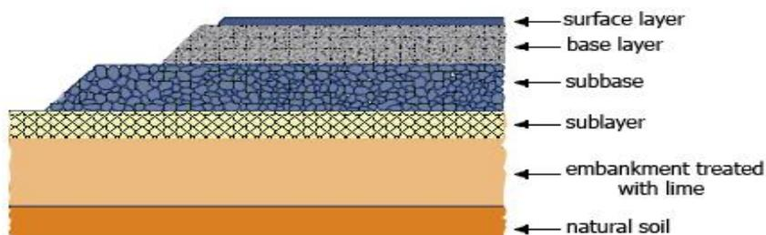
Figure 2. Cross section of the road
