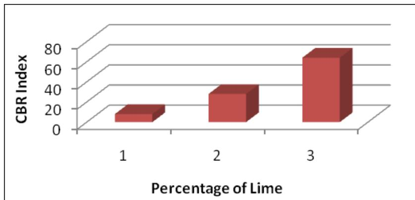
Figure 7. The CBR index based on the percentage of lime
