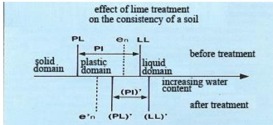
Figure 1. Immediate change of behavior of a moist clay soil caused by the introduction of the quicklime.
