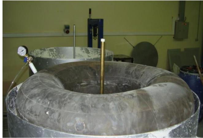
Figure 2. A large size inner tube used as an airbag placed in the tank to apply pressure
