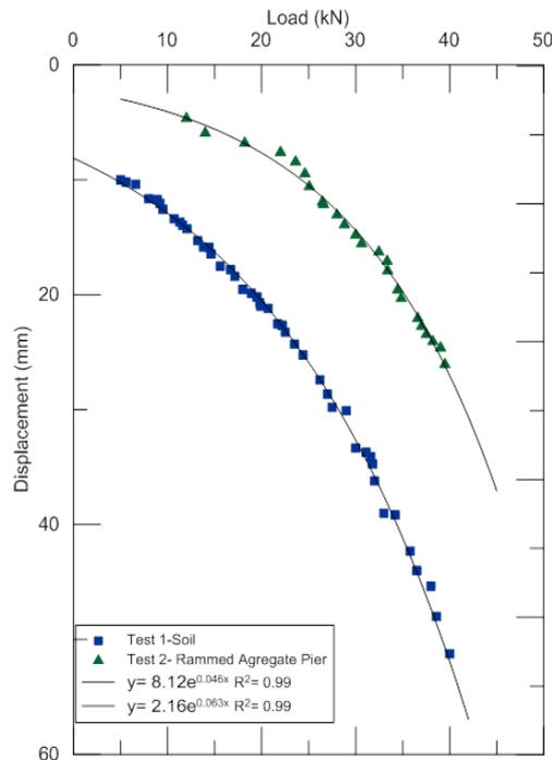
Figure 5. Load-displacement behavior of soil with and without RAP
