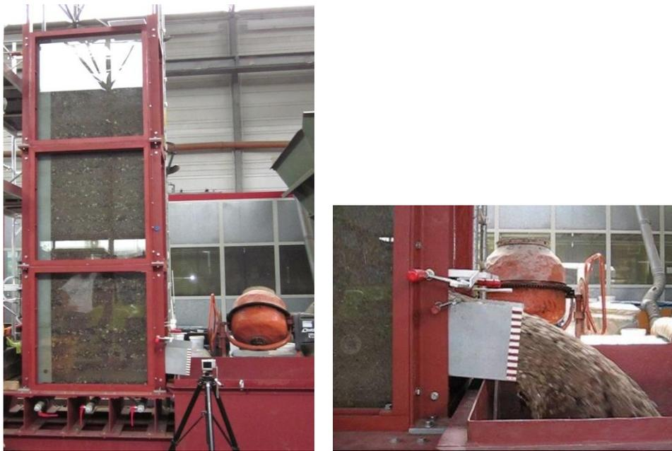
Figure 5. Filled test stand (left) and outflow during the test procedure (right)
