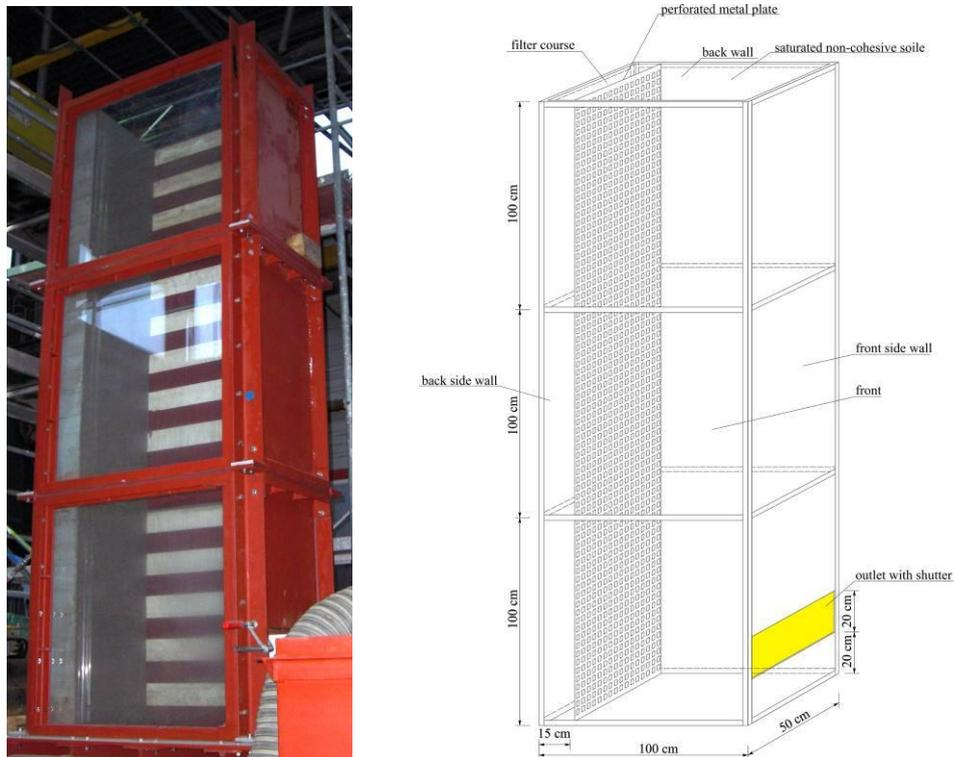
Figure 2. Experimental rig to analyse the flow behaviour of a fluid-granulate mixture
