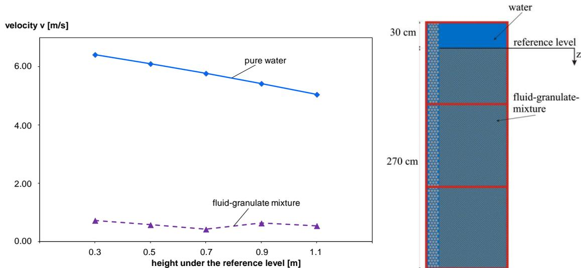
Figure 6. Velocity depending on the height under the reference level
