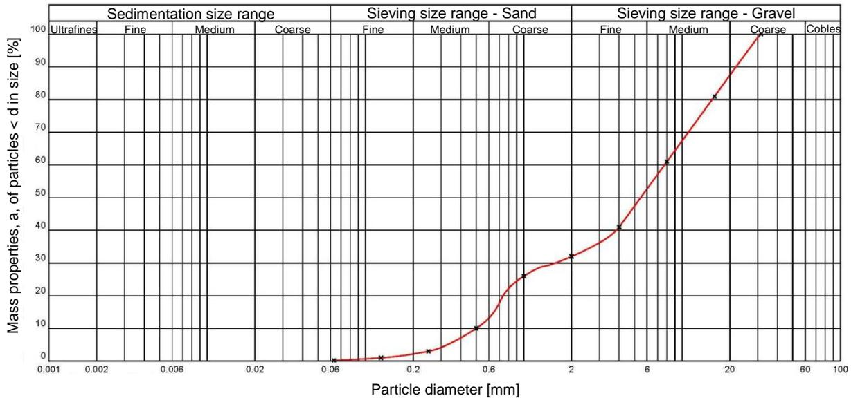
Figure 3. Grain-size distribution curve of the test material
