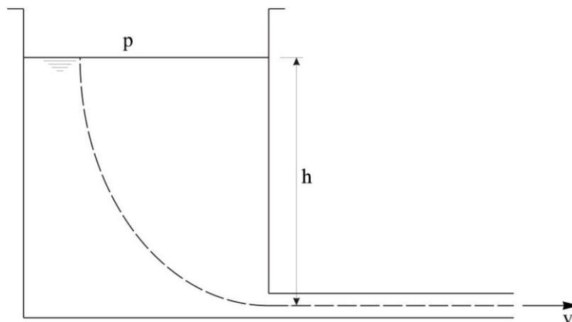
Figure 1. Outflow of a incompressible fluid out of a container
