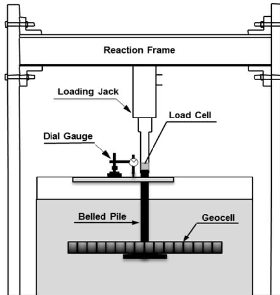
Figure 2. General arrangements of testing system.
