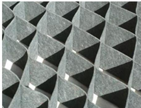
Figure 1. Isometric view of the Geocell.
