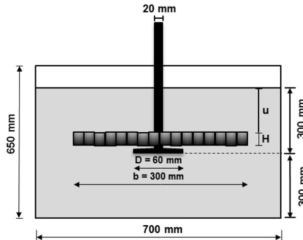
Figure 3. Geometry of the belled pile and Geocell reinforced foundation bed.
