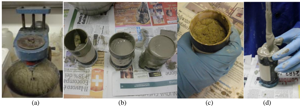
Figure 1. (a) Laboratory vane; (b) molding phases with No Compaction; (c) Tapping and (d) Rodding.
