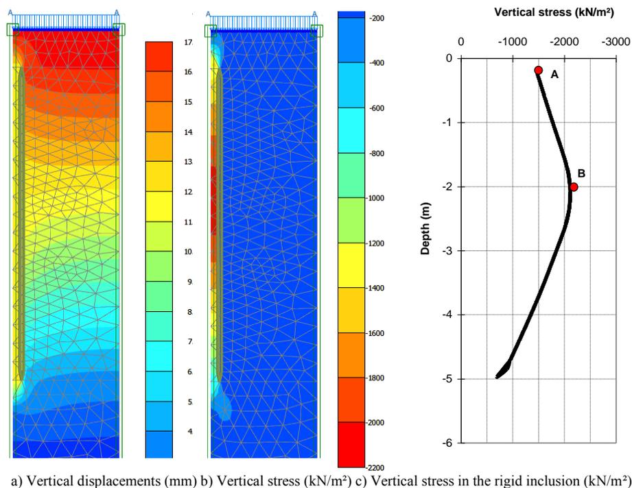
Figure 8. Vertical displacements and stresses after loading
