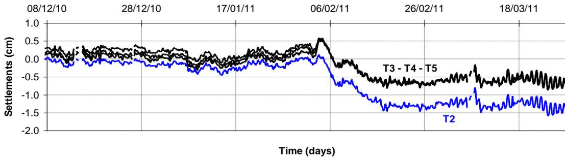
Figure 6. Settlement under the centre of the water concrete tank
