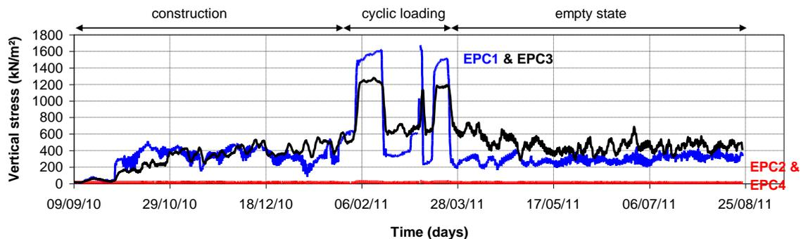
Figure 5. Stress distribution at inclusion head and soil
