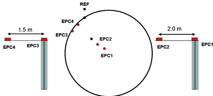
Figure 4. Location of earth pressures cells
