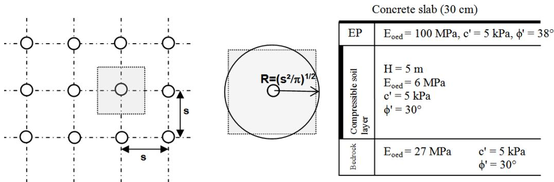
Figure 7. Characteristics of the soil layers and geometry used in the FEM Analysis
