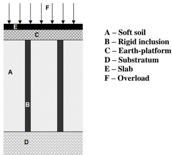
Figure 1. Soil reinforcement with rigid inclusions (Okyay, 2010).
