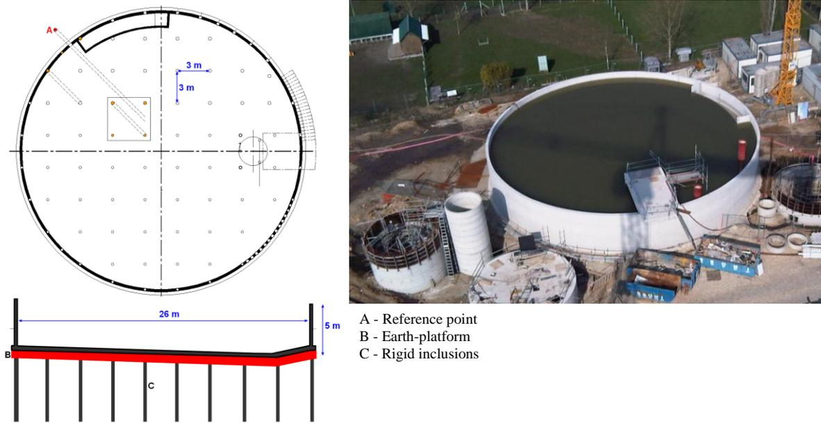
Figure 2. Plan and final views of the structure
