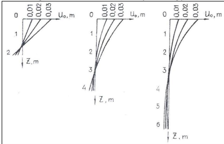
Figure 2. the elastic lines of piles.
