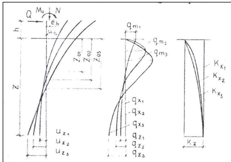
Figure 1. Analysis diagram for a laterally loaded pile.
