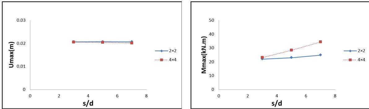
Figure 11: Effect of s/d on the maximum value of deflection and moment developed on piles
