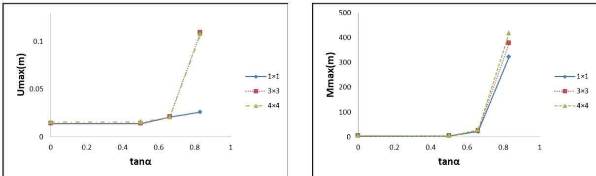
Figure6: Effect of angle of soil slope on the deflection and moment of piles in nxn square group
