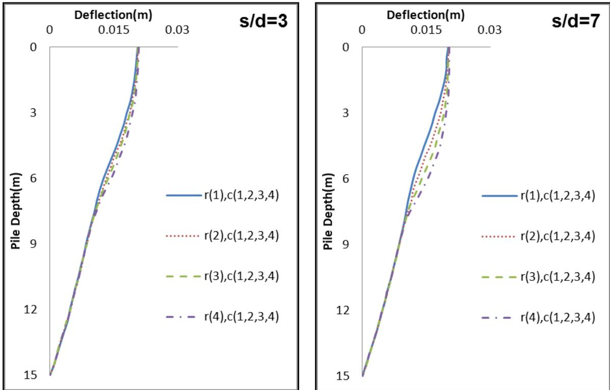
Figure9: Effect of  $s/d$  on the deflection of piles in  $4 \times 4$  square group
