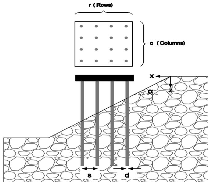
Figure2: The selected parameters for parametric study
