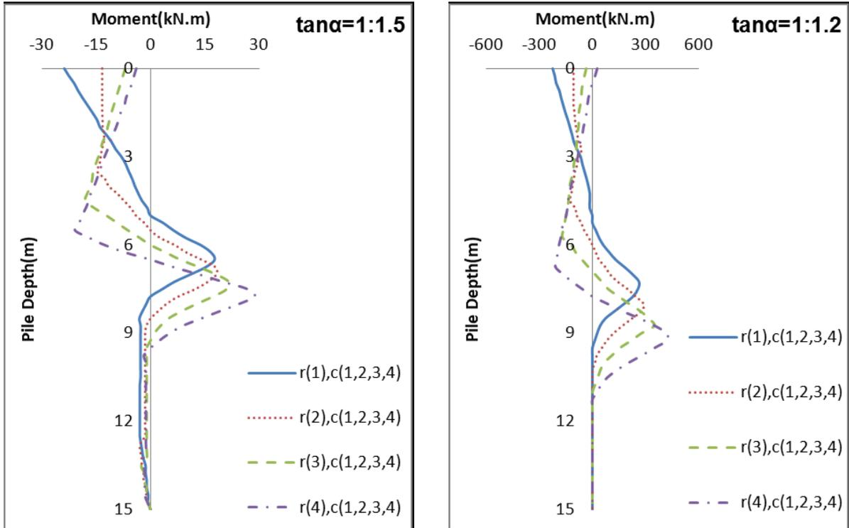
Figure5: The bending moment of 4x4 pile groups in 2 different angles of slopes
