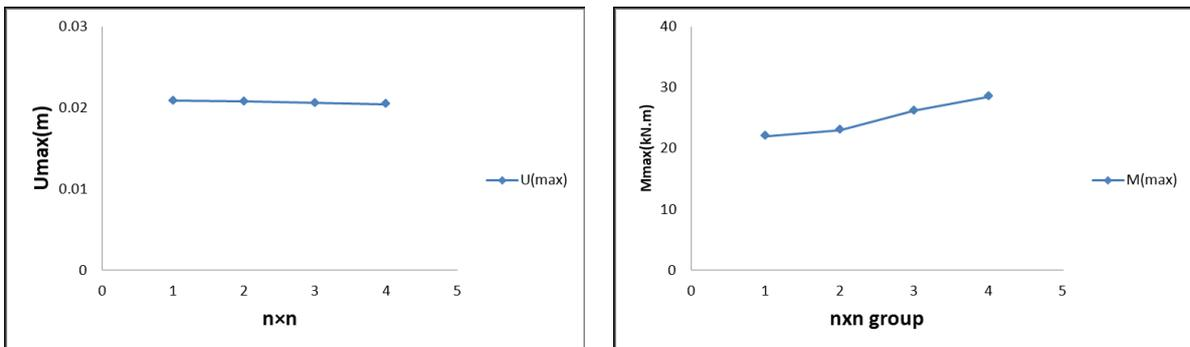
Figure8: The maximum value of deflection and moment developed on piles in n x n groups
