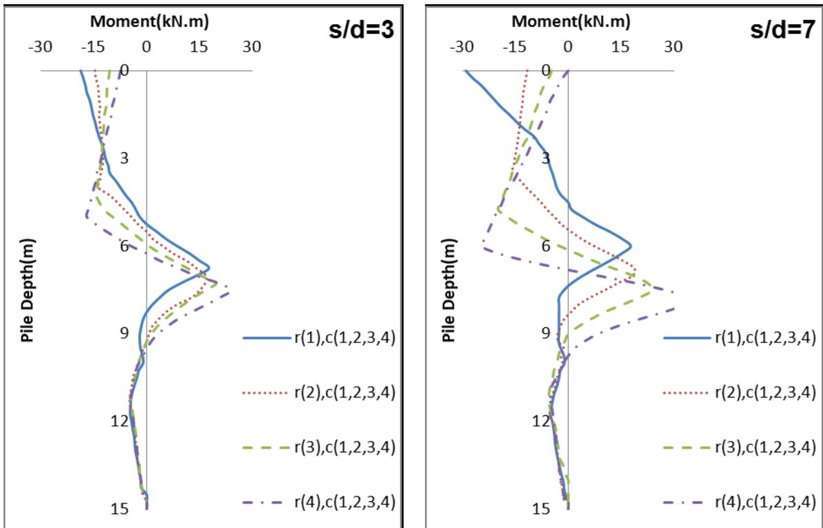
Figure10: Effect of  $s/d$  on the bending moment of piles in  $4 \times 4$  square group
