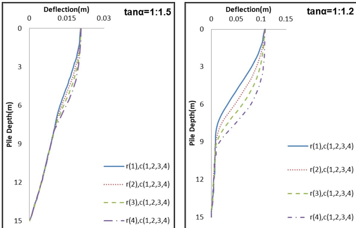
Figure4: The deflection of 4×4 pile groups in 2 different angles of slopes
