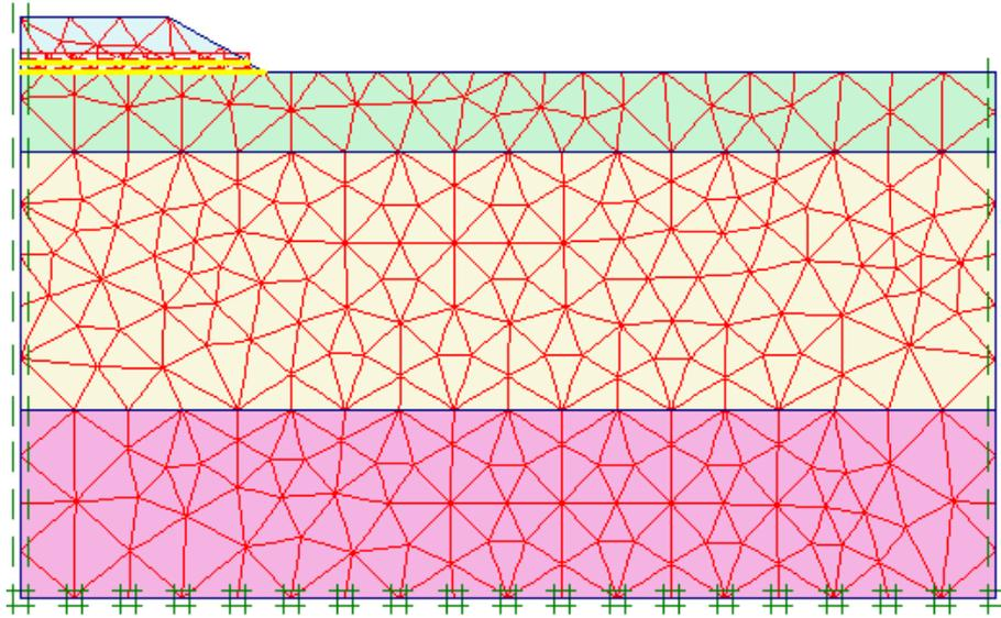
Figure 4. Finite element mesh of the embankment and foundation soil.
