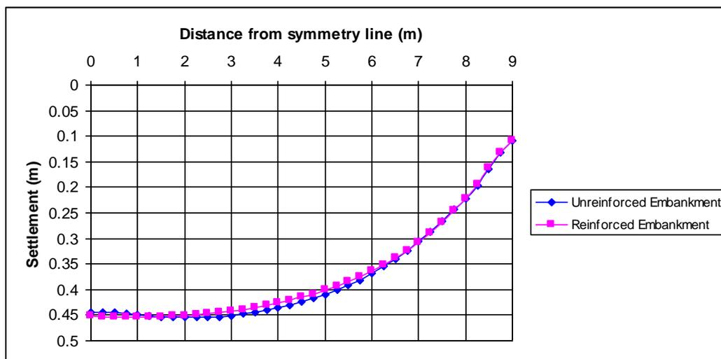
Figure 5. Effect of reinforcement on the settlement.
