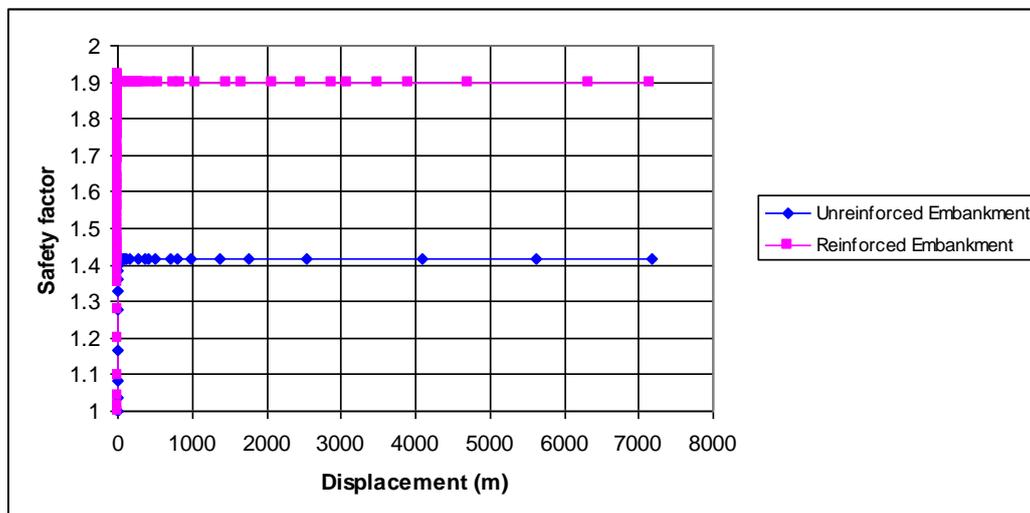
Figure 7. Safety factor of the embankment at the end of construction.
