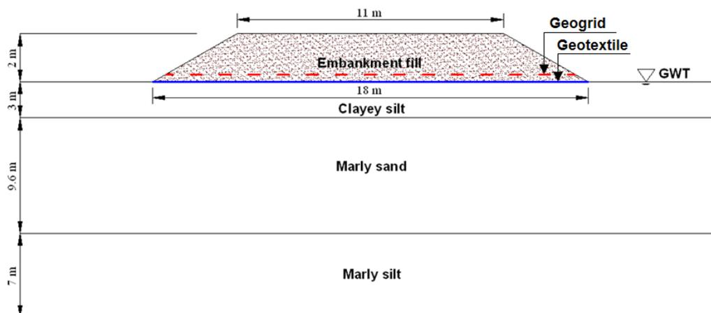
Figure 3. Generalized embankment geometry and foundation soil stratigraphy.
