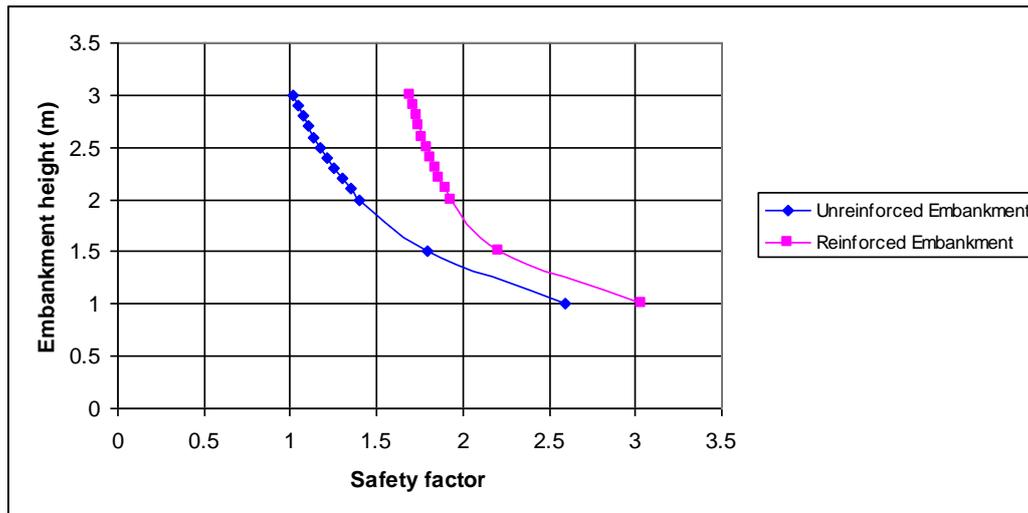
Figure 8. Effect of reinforcement on the embankment height.
