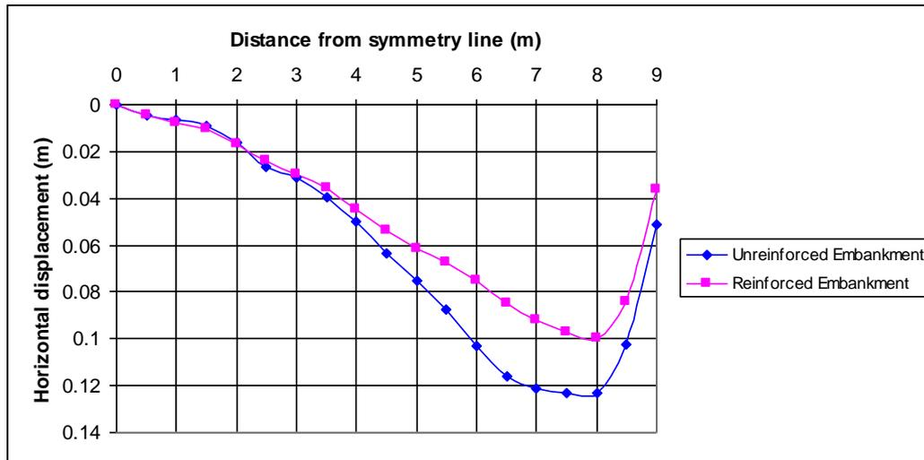
Figure 6. Effect of reinforcement on the horizontal displacement.
