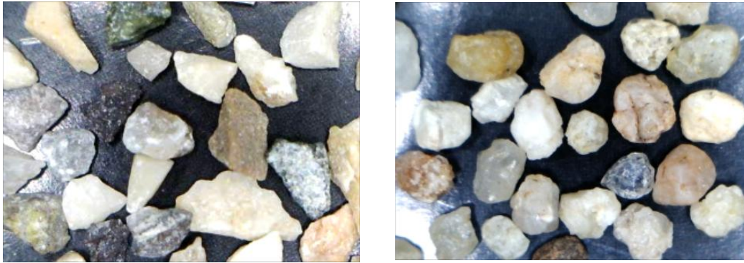
Figure 1. Picture of (a) crushed stone (Angular Sand: AS), and (b) Trakya (Rounded Sand: RS) sands used during the experimental study.
