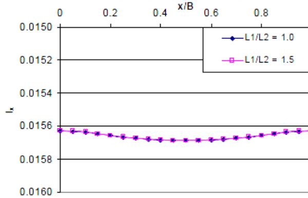
Figure 5. Normalized horizontal displacement of the piled-raft for different  $L_1/L_2$  ratios.
