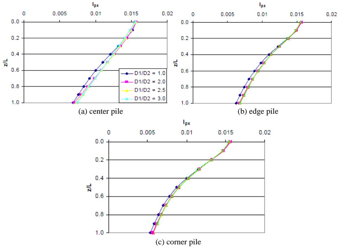
Figure 10. Normalized horizontal displacement along the pile at different pile locations for different  $D_1/D_2$  ratios.
