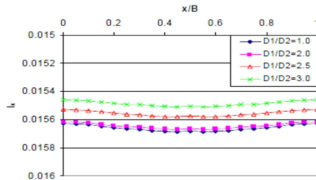
Figure 9. Normalized horizontal displacement of a piled-raft for different  $D_1/D_2$  ratios.
