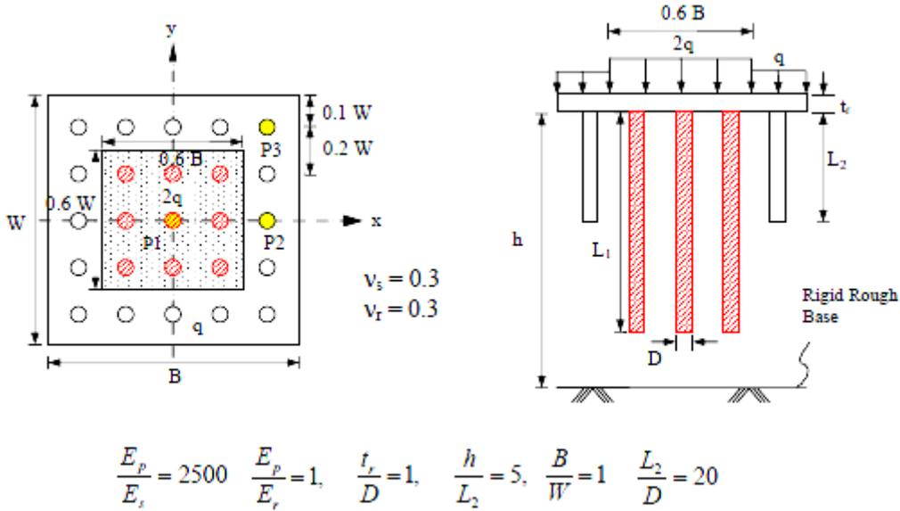
Figure 2. Configurations of the piled-raft.
