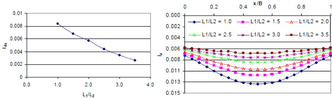
Figure 3. Variation of normalized differential and vertical displacement of the piled-raft with  $L_1/L_2$  ratios.
