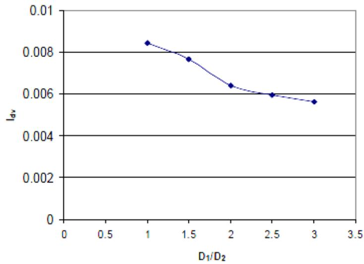
Figure 7. Variation of normalized differential displacement of the piled-raft with  $D_1/D_2$  ratios.
