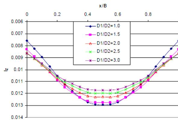
Figure 8. Normalized vertical displacement of the piled-raft for different  $D_1/D_2$  ratios.
