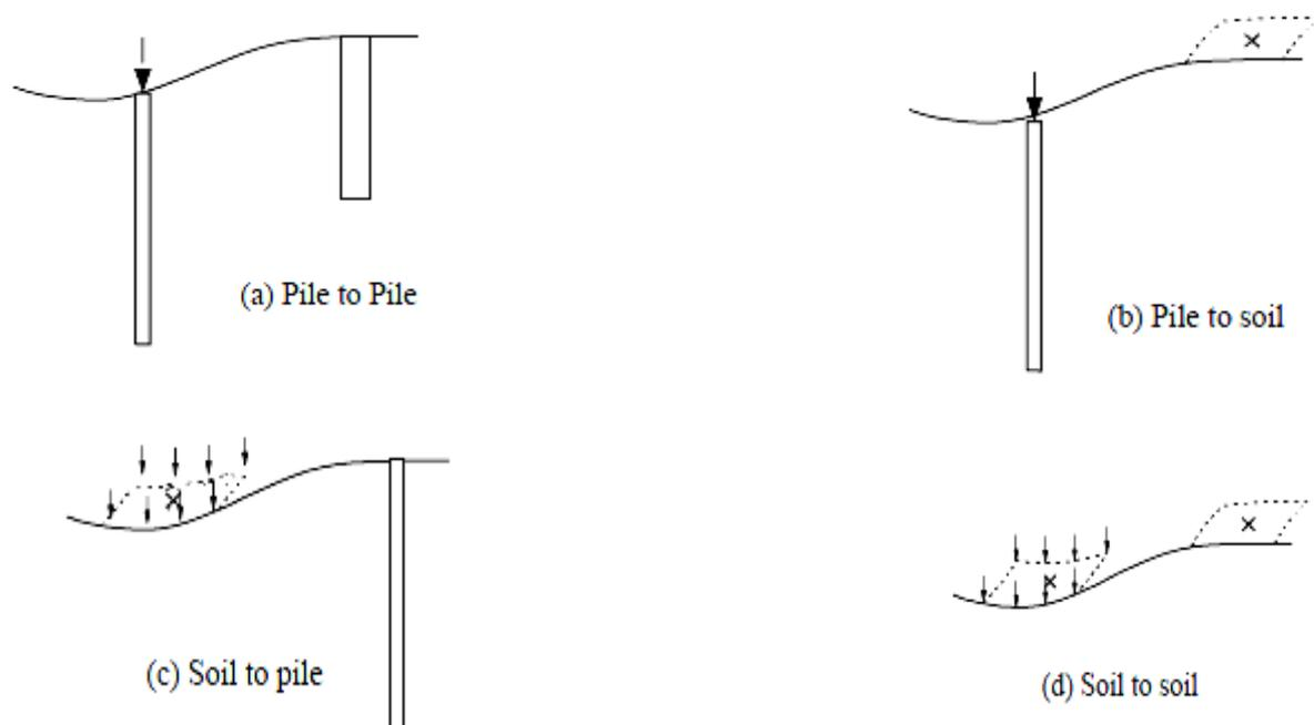
Figure 1. Types of interaction in piled-raft foundation.
