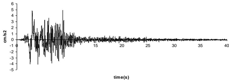
Figure 1. Acceleration time history of Bam earthquake (Mw=6.6).
