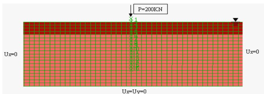
Figure 3. Numerical model of soil-pile system.
