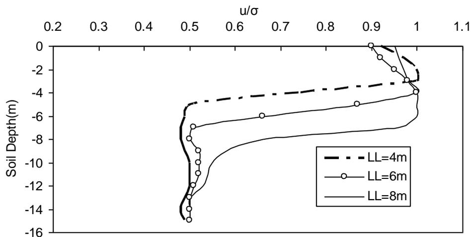
Figure 4. EPWPR for liquefied soil depths of 4 m, 6 m and 8 m ( $D_r=45\%$ ).
