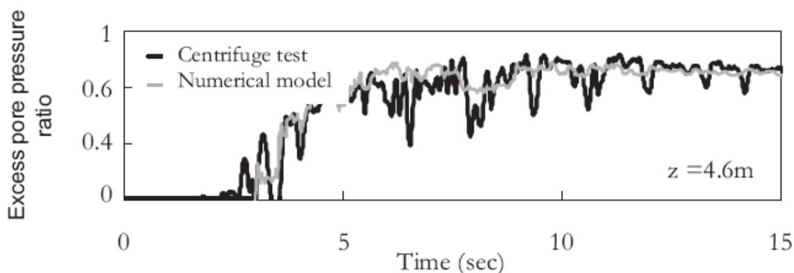
Figure 2. Comparison of excess pore water pressure ratio time history from the test and numerical model (after Haldar & Babu, 2010).
