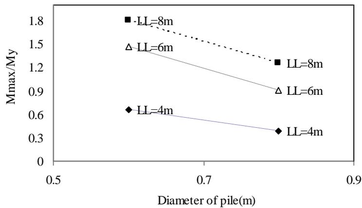
Figure 5.  $M_{max}/M_y$  ratio for different liquefied depths and pile diameters.
