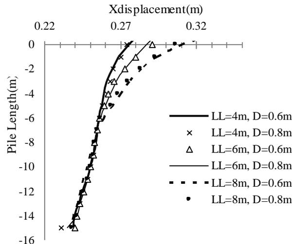
Figure 6. Maximum lateral pile displacement obtained from the numerical model.
