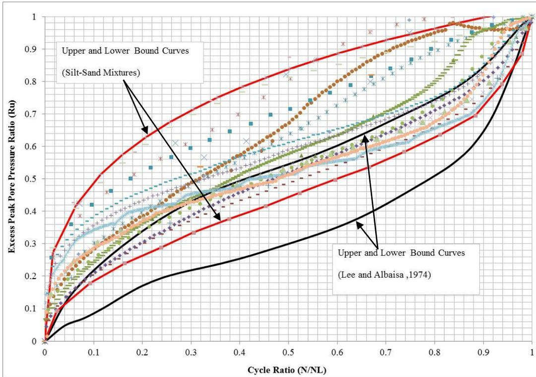
Figure 3. Maximum and minimum peak pore pressure generation in sand and silt mixture specimens over a wide range of parameters and compared with Lee and Albaisa (1974)
