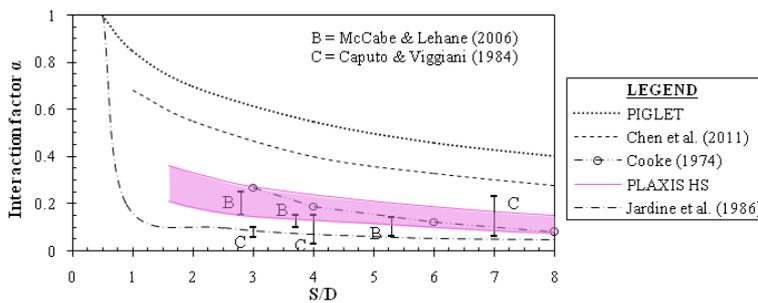
Figure 5. Comparison of interaction factor predictions to field data
