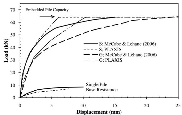
Figure 4. Predictions of single pile and pile group response using embedded piles compared to field data
