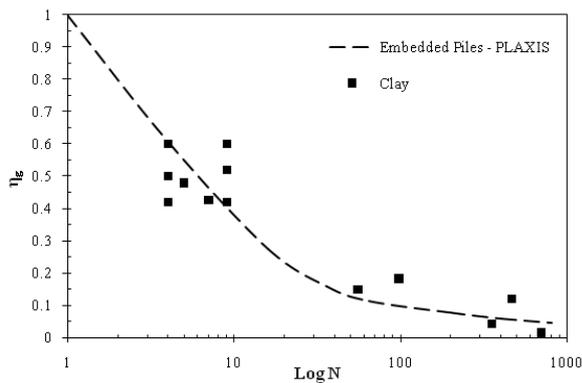
Figure 8. Comparison of stiffness efficiency predictions to field data
