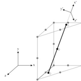
Figure 1. Illustration of beam element (pile) crossing 15-node wedge element (Brinkgreve, 2007)
