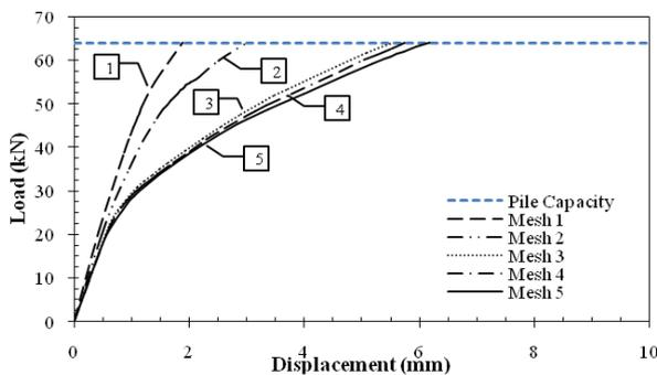
Figure 3. Results of the different FE meshes
