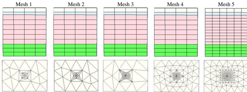
Figure 2. The FE meshes used in the 3-D analyses
