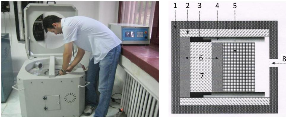
Figure 2. The small geotechnical centrifuge employed for the present investigation (left) and the schematical cross section of the centrifuge consolidation cell (right): 1) Fixed housing to hold the test specimen, 2) inner cylindrical module, 3) consolidation ring (D=50 mm, h=20 mm), 4) centralizer, 5) surcharge, 6) porous stone, 7) soil specimen, 8) laser beam entry hole (dimensions are proportional to consolidation ring).
