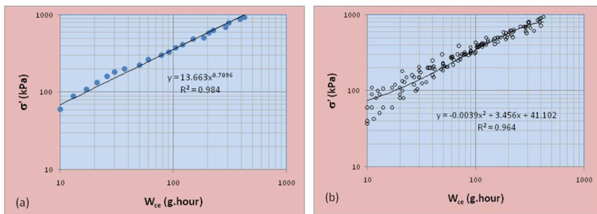
Figure 3. Plot of the effective stress versus the equivalent centrifuge load data: (a) from Figure 1; (b) for 8 artificially consolidated soils. Each point on graphs corresponds to certain axial strain.
