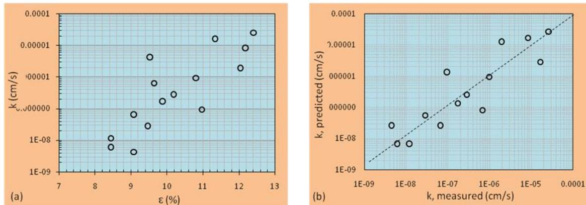
Figure 5. Correlation between the coefficient of permeability from falling-head test methods and axial strains from the centrifuge consolidation tests (a) and correlation between predicted and measured permeabilities (b).
