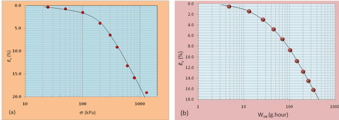
Figure 1. Sample plots for consolidation tests. (a) Conventional oedometer; (b) centrifuge consolidation (the results belong to the specimens artificially consolidated at 600 RPM).
