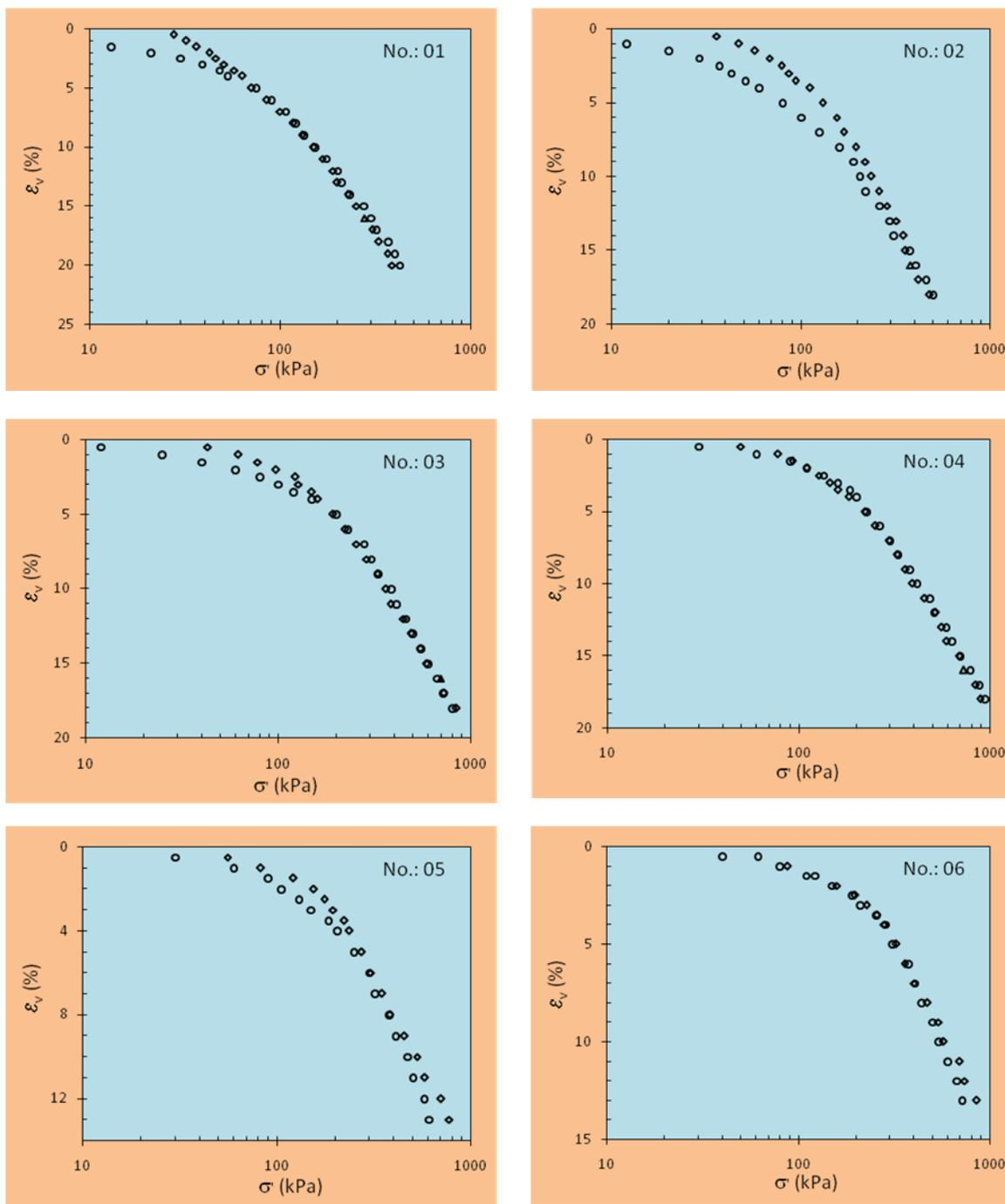
Figure 4. Comparison between the results from conventional consolidation tests (circles) and the predicted effective stresses (diamonds) from the centrifuge consolidation data using the conversion equation.
