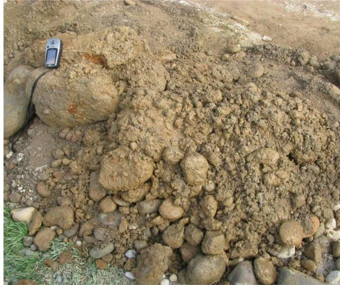
Figure 4. A picture of cobbles and boulders in the middle of TML2 (Daneshsara square)
