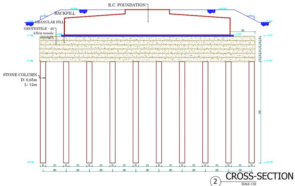
Figure 10. Cross-section of stone column application on a turbine.
