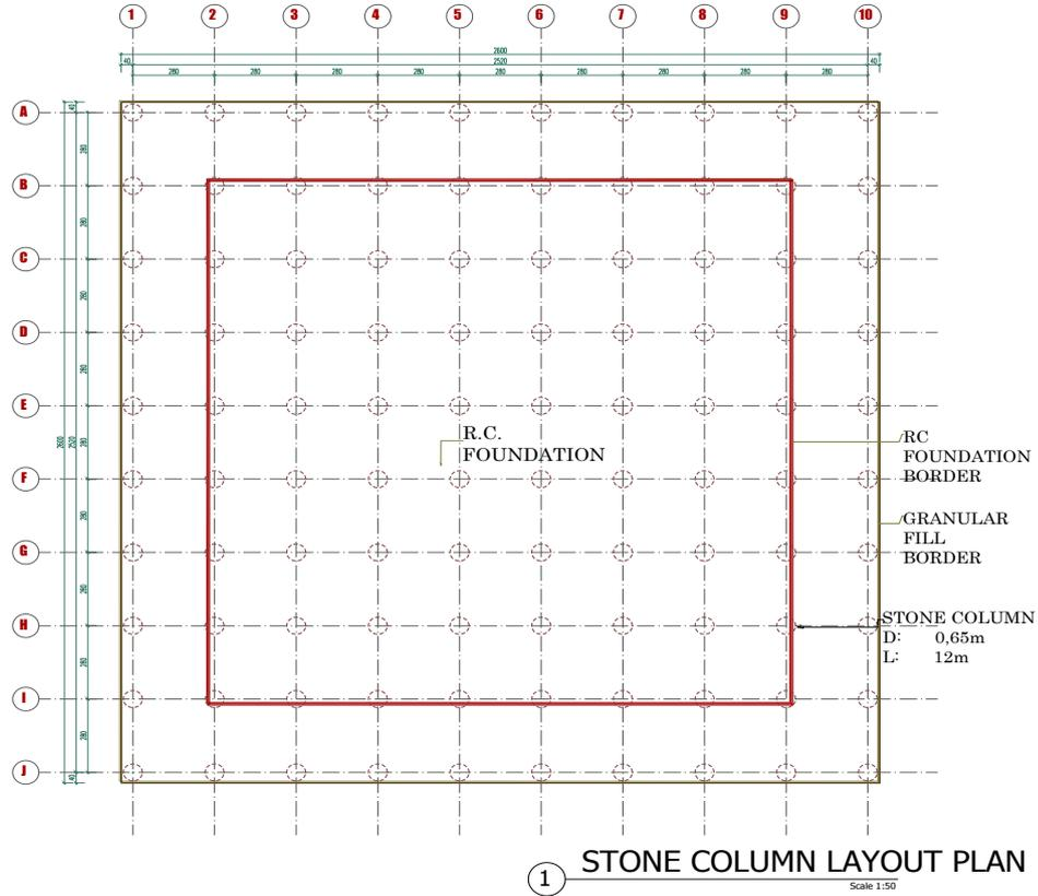
Figure 9. Stone column layout plan for a turbine foundation.
