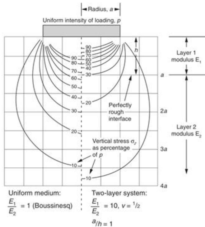
Figure 1. Westergaard stress distribution for a two-layer system (Munfakh et al., 2001).
