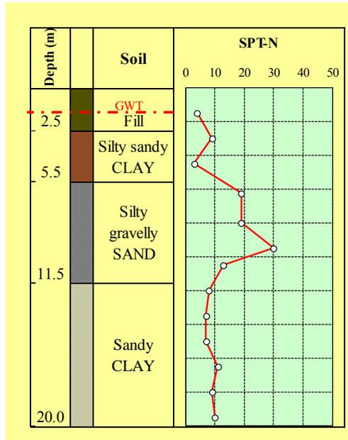
Figure 2. Soil profile based on the subsurface borings.
