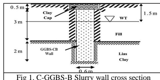
These walls are constructing by low permeation material to reduce the groundwater streams into the encapsulated area to preclude contaminant migration in the way of groundwater. The most common type of self hardening slurry material; Cement-bentonite (CB) are typically limits the hydraulic
