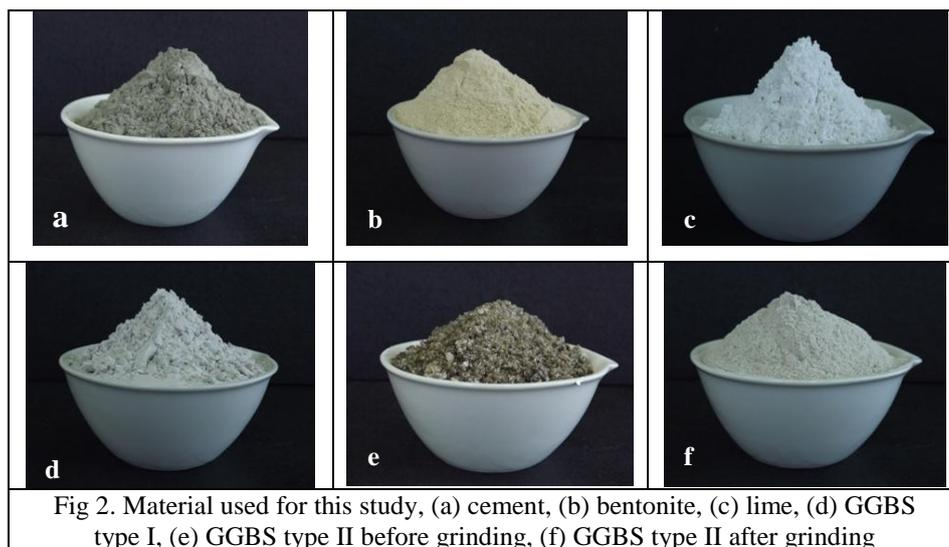
Fig 2. Material used for this study, (a) cement, (b) bentonite, (c) lime, (d) GGBS type I, (e) GGBS type II before grinding, (f) GGBS type II after grinding
