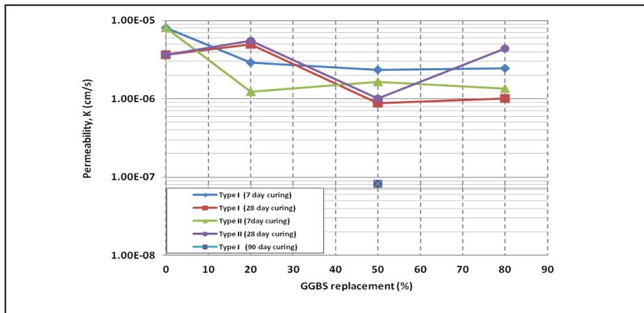
Fig. 3. Permeability of both GGBS cured for 7 and 28 days.
