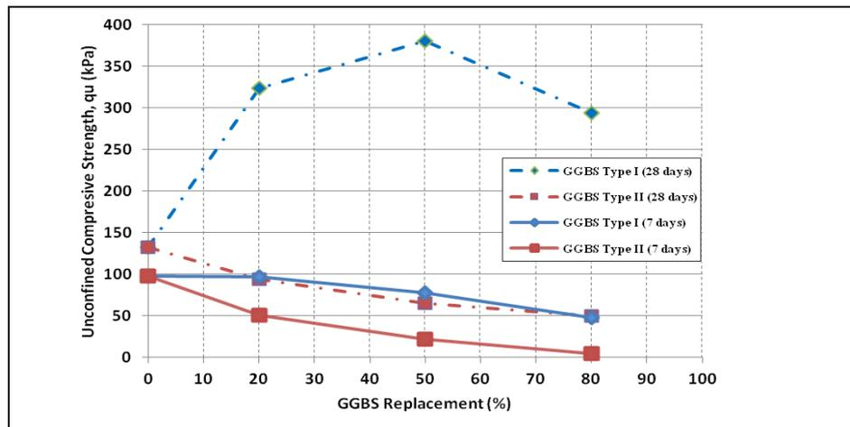
Fig. 4. Unconfined compressive strength of both GGBS (bentonite content 5%)
