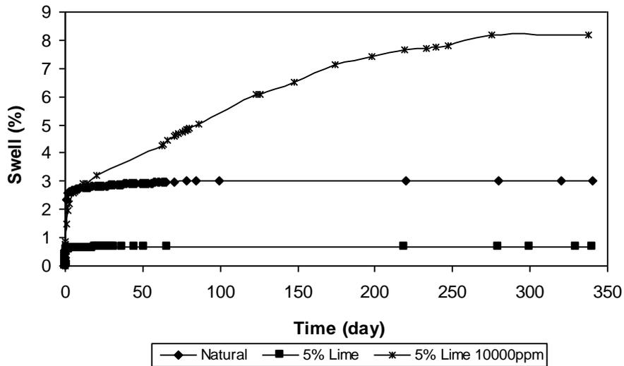
Figure 1. Swell percent of the control soil, 5% lime stabilized soil and 5% lime stabilized soil subjected to 10000 ppm sulfate solution.
