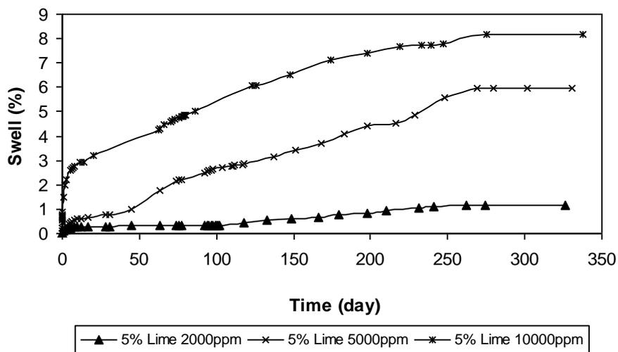
Figure 2. Swell percentage of 5% lime stabilized soil subjected to different concentration of sulfate solutions: 2000, 5000 and 10000 ppm.
