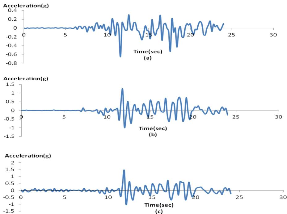
Figure 3. Time-acceleration on the ground: (a) dense, (b) medium and (c) loose sand
