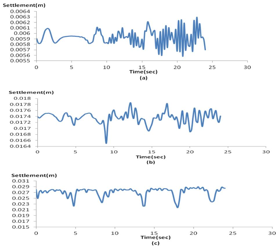
Figure 5. Settlement of the tank in: (a) dense, (b) medium and (c) loose sand
