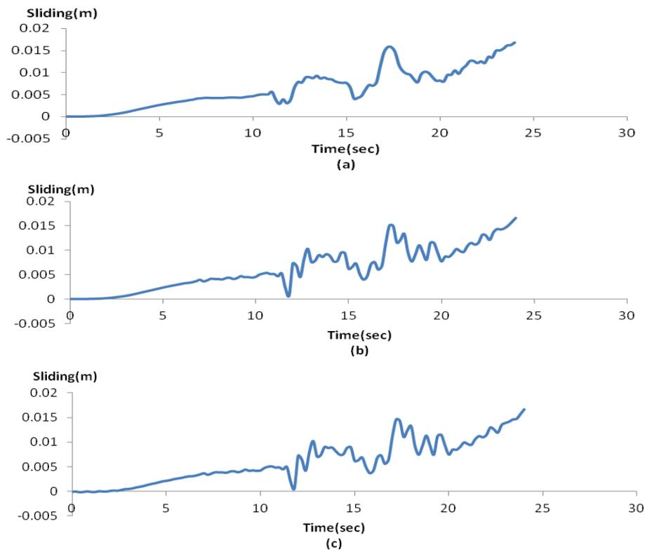
Figure 4. Sliding of the tank in: (a) dense, (b) medium and (c) loose sand
