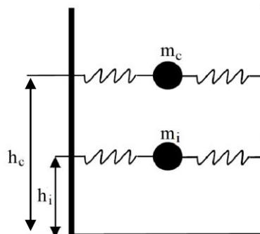
Figure 1. Simplified Mass Spring Model (MSM) proposed by Malhotra et al. (2000).
