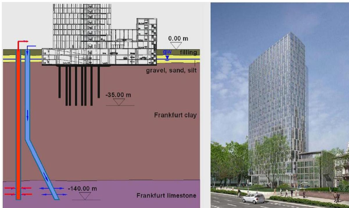
Figure 2. Heating/cooling system of WestendDuo, Frankfurt
