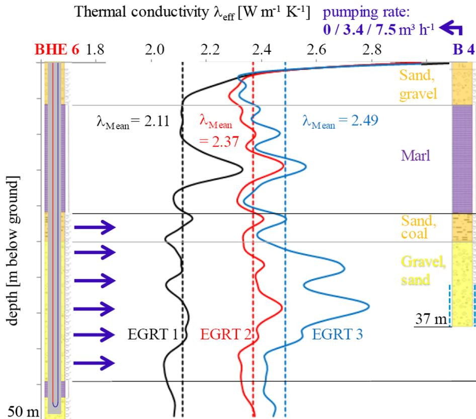
Figure 5. Effective thermal conductivity over depth
