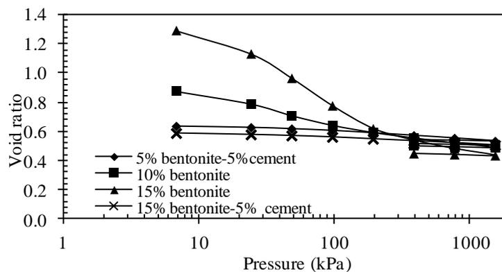
Figure 3. Consolidation test results.
