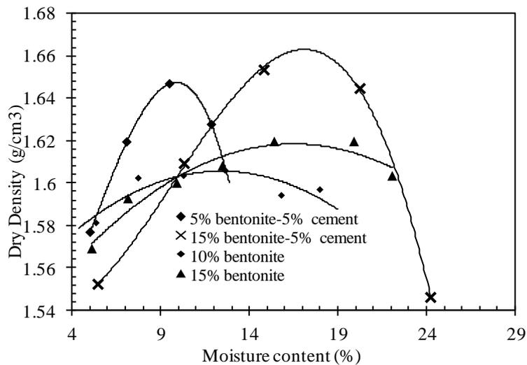
Figure 1. Compaction curves.
