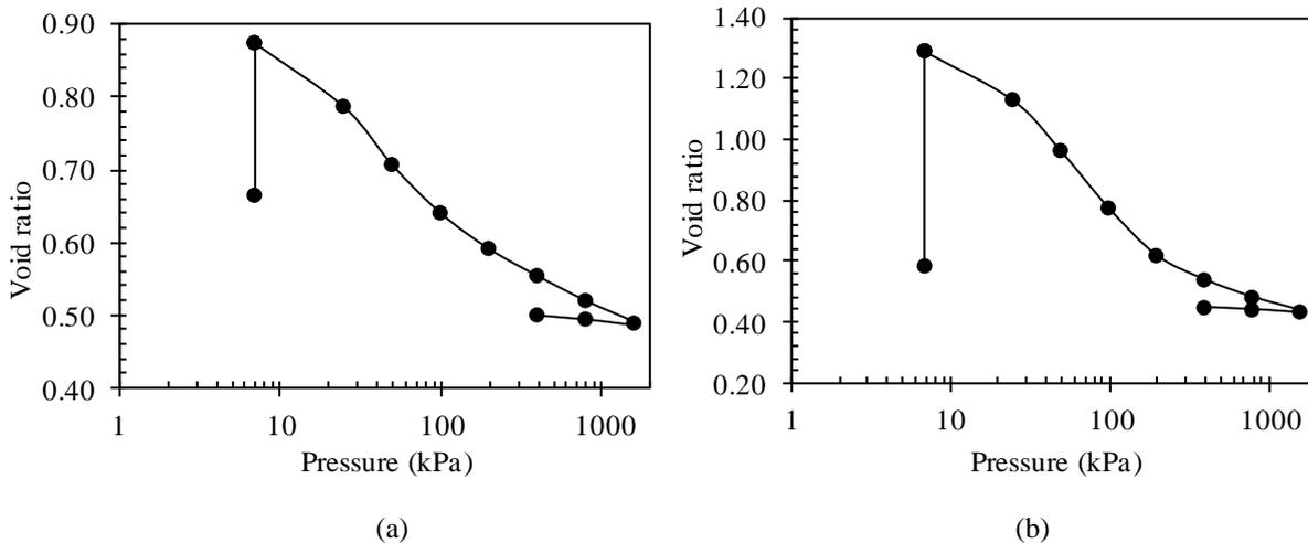
Figure 4. Consolidation curves of (a) 15% bentonite and, (b) 10% bentonite samples.
