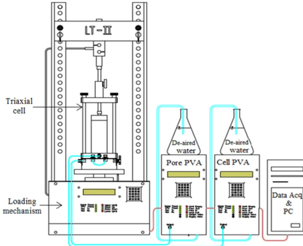
Figure 3. Schematic view of triaxial system (adopted from Geocomp, 2010)
