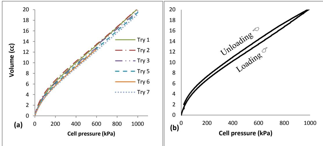
Figure 4. Calibration cycles with gradual loading/unloading.
