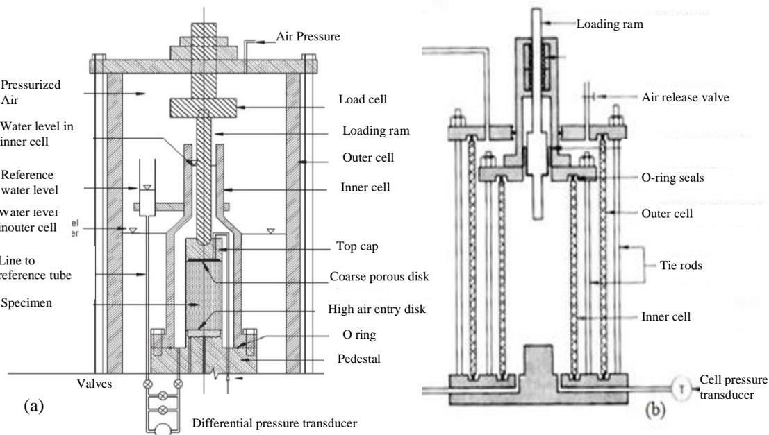
Figure 1. Double wall volume measuring triaxial setup a) (Ng et al. 2002) b) (Wheeler 1988)
