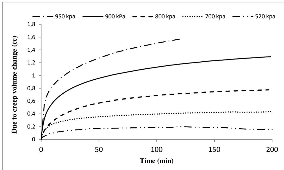
Figure 5. Creep behavior under constant pressure. Time axis starts from the end of pressurization
