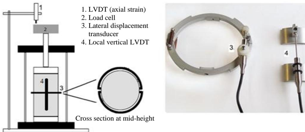
Figure 2. Local strain gauges for measuring of sample volume change in a triaxial apparatus
